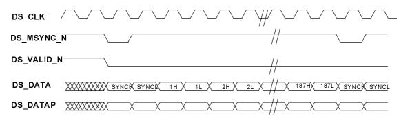
Figure F-3: Downstream Data Signal Protocol for annex B Operation
