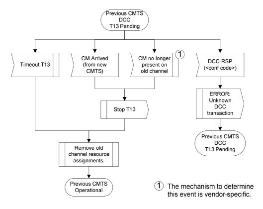
Figure 11-44: Dynamically Changing Channels: CMTS View Part 3
