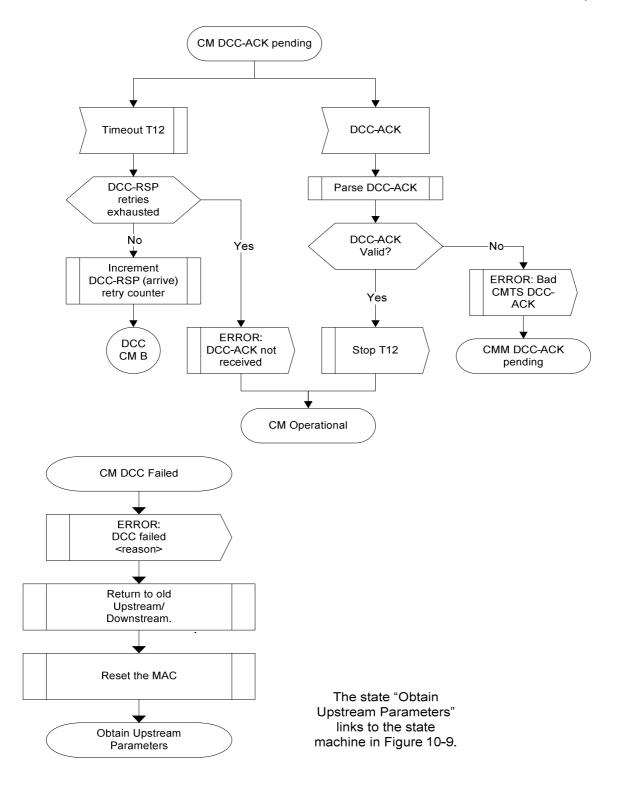
Figure 11-49: Dynamically Changing Channels: CM View Part 4
