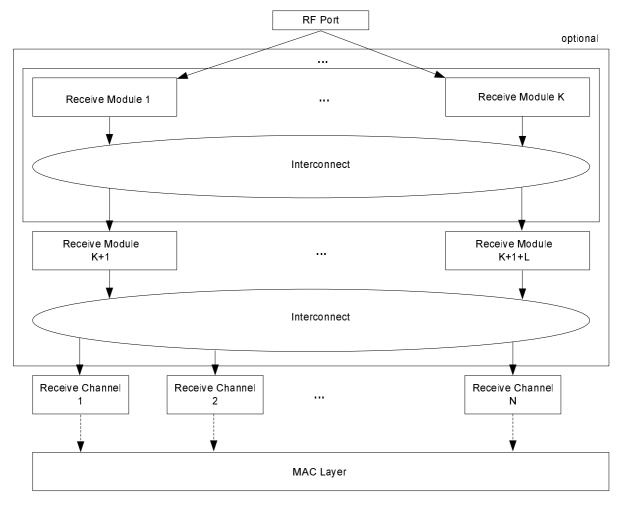
Figure 8-1: Interconnection between Receive Channels and Receive Modules
