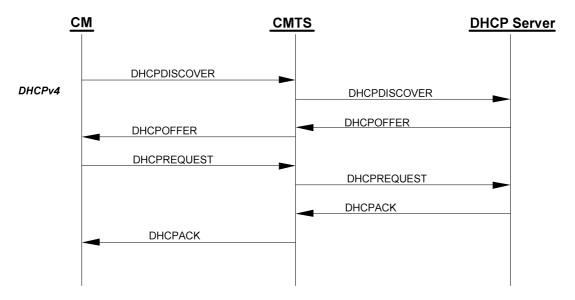
Figure 10-23: IPv4 Provisioning Message Flow
