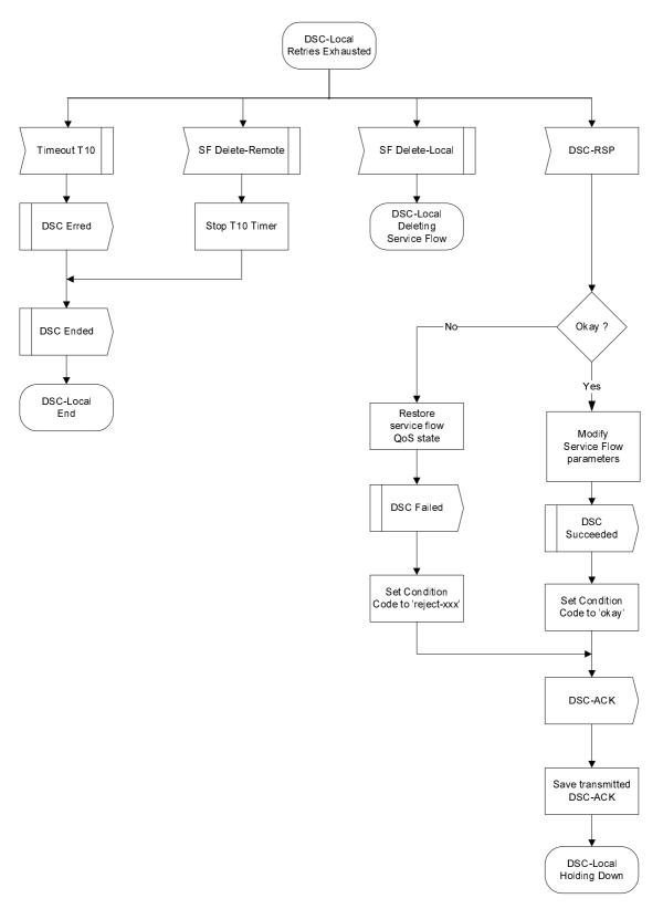
Figure 11-26: DSC-Locally Initiated Transaction Retries Exhausted State Flow Diagram
