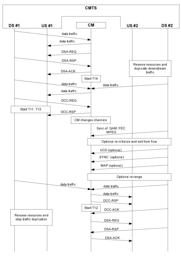
Figure W-1: DCC Example Operational Flow
