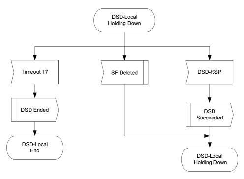
Figure 11-36: DSD-Locally Initiated Transaction Holding Down State Flow Diagram
