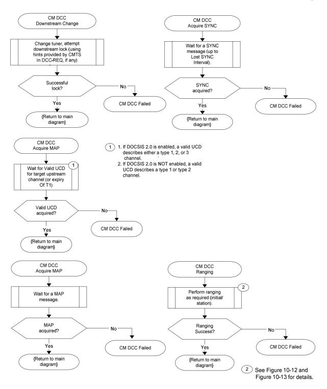
Figure 11-48: Dynamically Changing Channels: CM View Part 3
