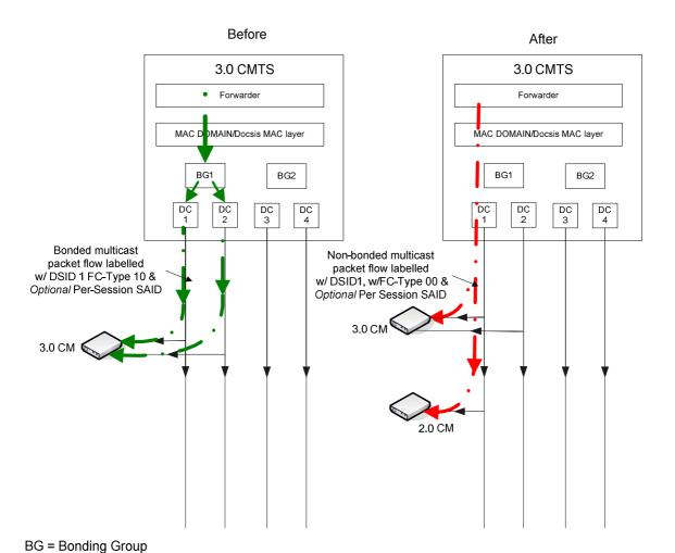
Figure S-4: Multicast Session Replication to clients behind both a 3.0 CM and a 2.0 CM on the same downstream channel (Subcase 1)
