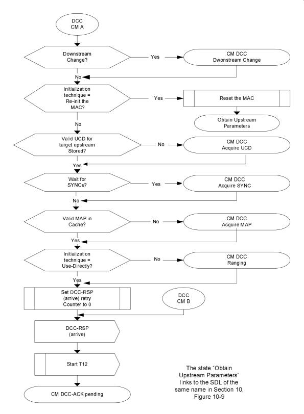
Figure 11-47: Dynamically Changing Channels: CM View Part 2
