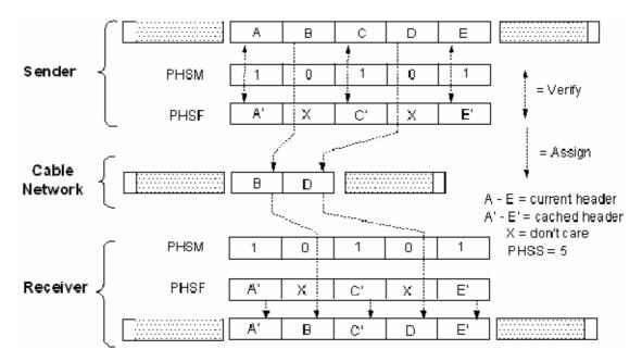
Figure 7-19: Payload Header Suppression with Masking
