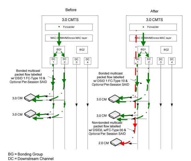
Figure S-5: Bonded and Non-bonded replications of a Multicast Session on an overlapping downstream channel using FC 10 Isolation Technique (Subcase 2)
