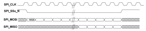
Figure F-7: SPI Bus Transaction
