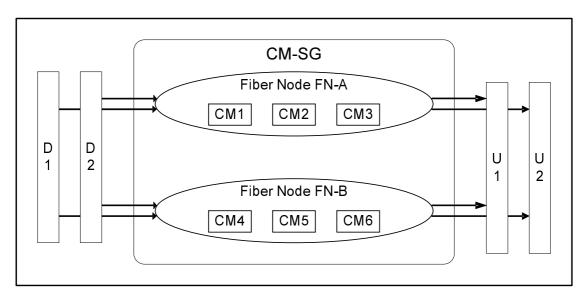
Figure 5-7: Multiple fibre nodes per CM-SG
