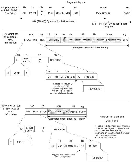
Figure 7-8: Example of Fragmenting a Single Packet
