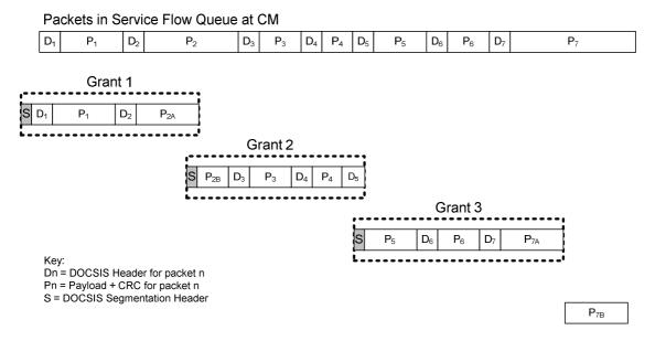
Figure 7-4: CCF using Segment Headers
