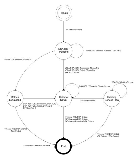
Figure 11-3: DSA-Locally Initiated Transaction State Transition Diagram
