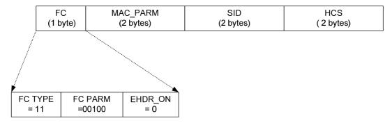
Figure 6-9: Queue-depth Based Request Frame Format
