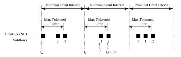
Figure O-1: Example Jitter with Multiple Grants per SID
