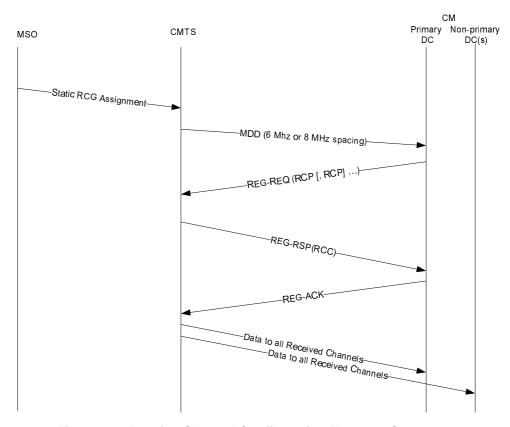
Figure 8-3: Receive Channel Configuration Message Sequence
