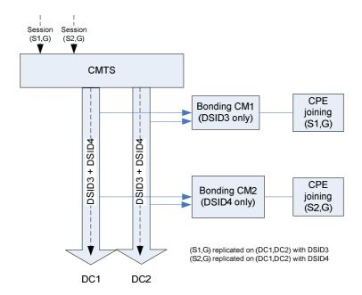
Figure 9-4: DSIDs separate Source-Specific Multicast Sessions
