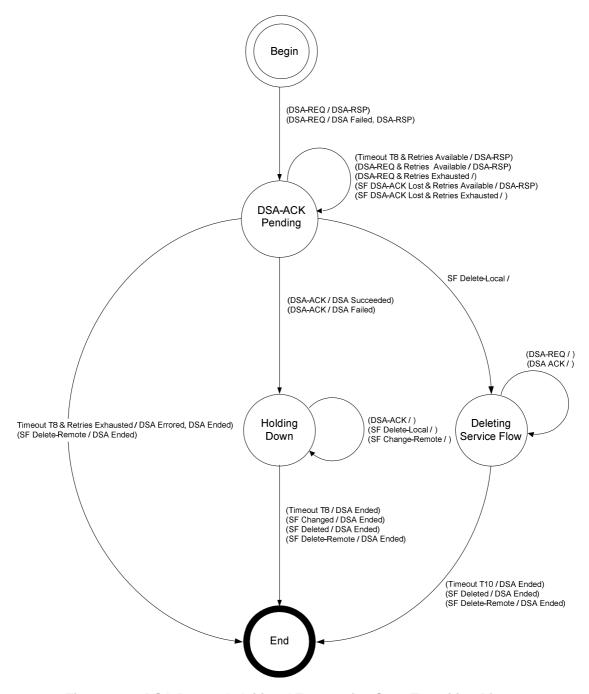
Figure 11-4: DSA-Remotely Initiated Transaction State Transition Diagram
