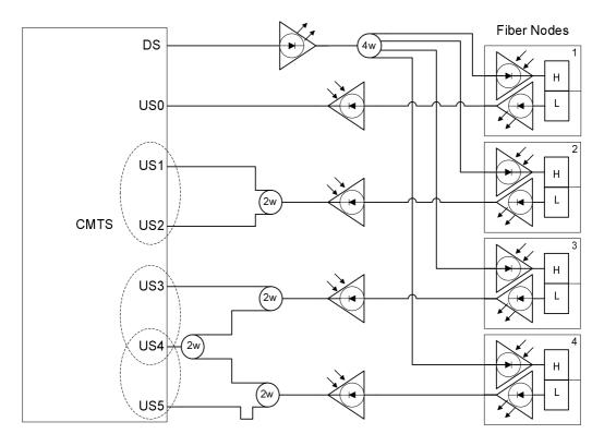
Figure W-4: Example Combining Network 1
