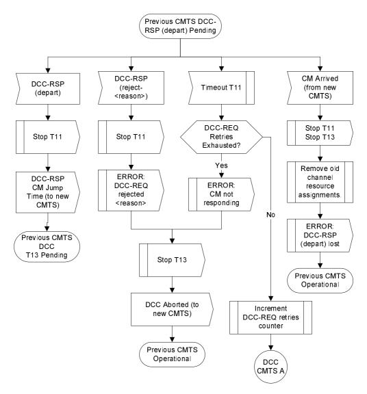
Figure 11-43: Dynamically Changing Channels: CMTS View Part 2
