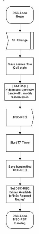
Figure 11-23: DSC-Locally Initiated Transaction Begin State Flow Diagram
