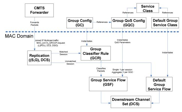
Figure 7-17: IP Multicast QoS Object Model Diagram
