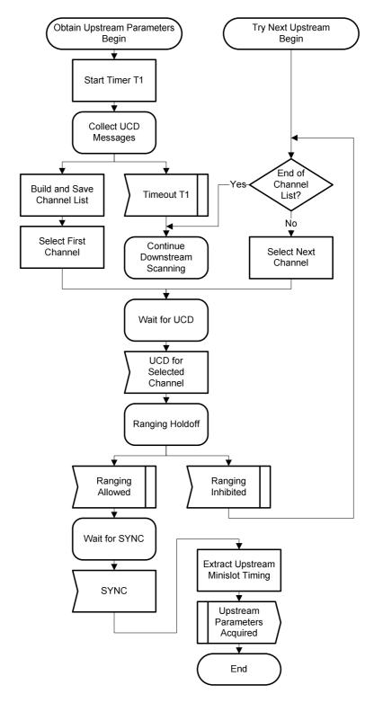
Figure 10-9: Obtain Upstream Parameters
