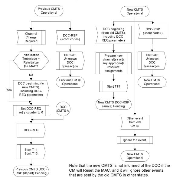
Figure 11-42: Dynamically Changing Channels: CMTS View Part 1
