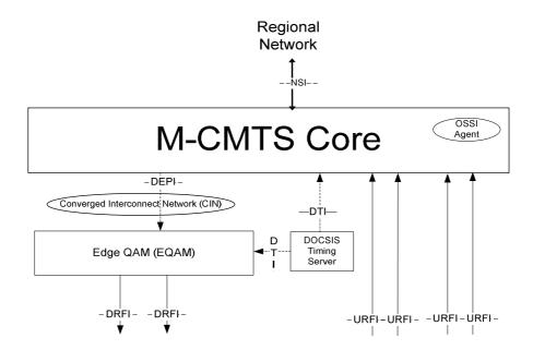
Figure 5-2: Modular CMTS Network Diagram
