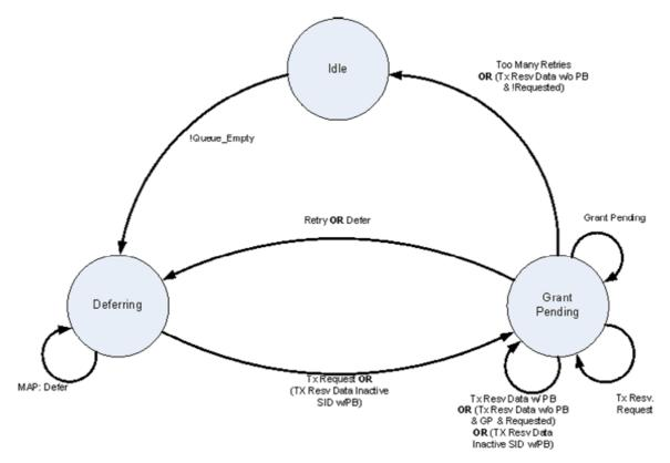
Figure N-1: Transmission and Deference State Transition Diagram (Multiple Transmit Channel Mode)
