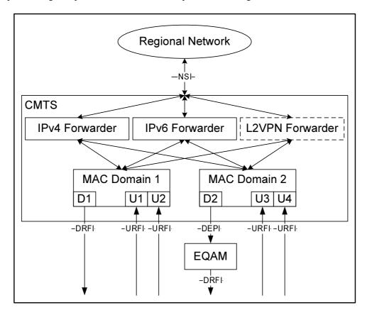
Figure 5-3: CMTS Internal Forwarding Model
