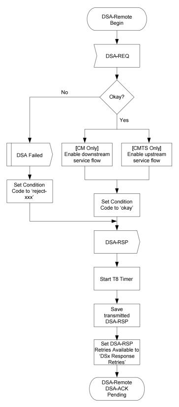
Figure 11-16: DSA-Remotely Initiated Transaction Begin State Flow Diagram
