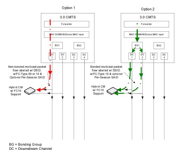
Figure S-2: Multicast Session Replication for a client behind a Hybrid CM capable of FC-Type 10
