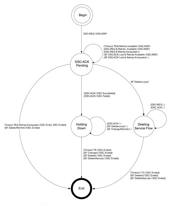
Figure 11-6: DSC-Remotely Initiated Transaction State Transition Diagram
