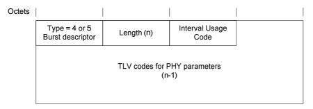
Figure 6-16: Top-Level Encoding for Burst Descriptors
