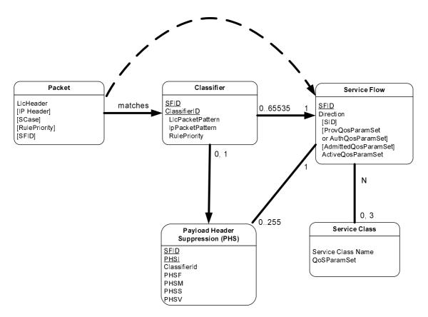
Figure 7-13: Theory of Operation Object Model
