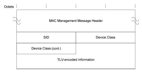
Figure 6-44: Device Class Identification Request
