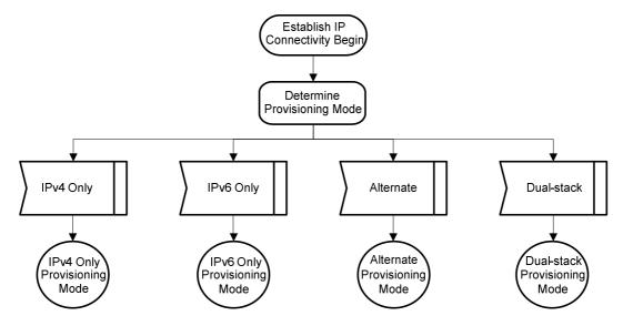
Figure 10-16: Establish IP Connectivity
