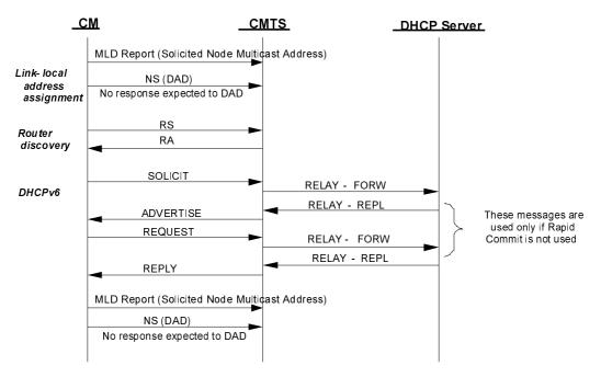
Figure 10-24: IPv6 Provisioning Message Flow
