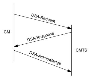
Figure 7-15: Dynamic Service Addition Message Flow - CM Initiated
