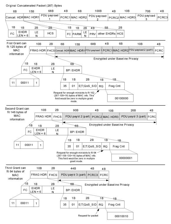
Figure 7-9: Fragmented Concatenated Packet Example
