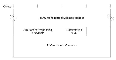
Figure 6-30: Registration Acknowledgment
