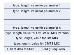
Figure D-6: Add End of Data Marker and Padding
