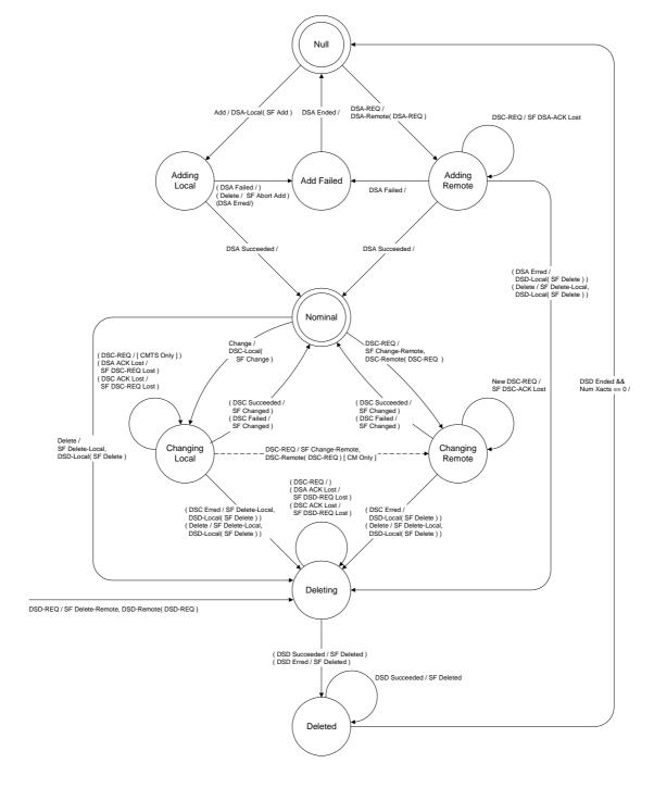
Figure 11-2: Dynamic Service Flow State Transition Diagram
