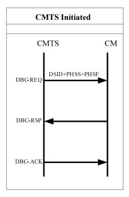
Figure 7-21: Signalling of a DSID-Indexed Payload Header Suppression Rule
