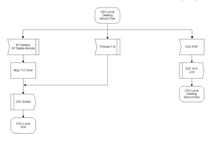
Figure 11-27: DSC-Locally Initiated Transaction Deleting Service Flow State Flow Diagram
