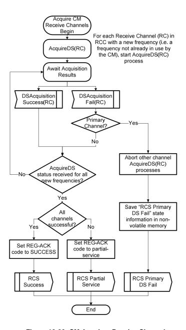
Figure 10-26: CM Acquires Receive Channels
