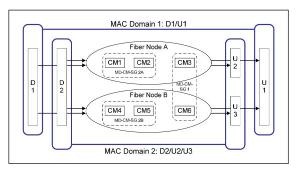
Figure 5-9: Multiple MAC Domains per Fibre Node
