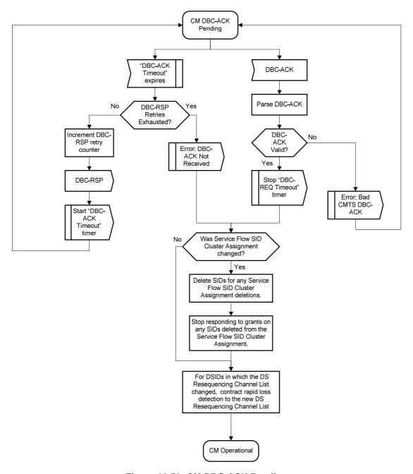
Figure 11-59: CM DBC-ACK Pending
