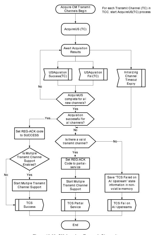
Figure 10-28: CM Acquires Transmit Channels
