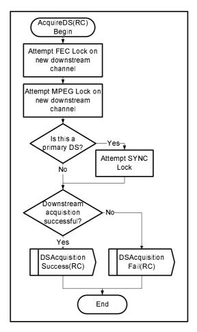
Figure 10-27: CM Acquires Downstream Channels
