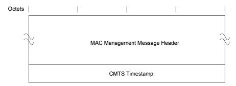
Figure 6-14: Format of Packet PDU Following the Timing Header
