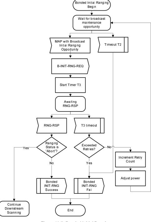
Figure 10-7: Bonded Initial Ranging
