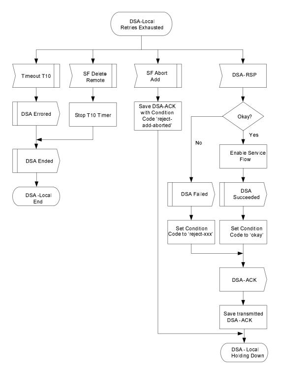
Figure 11-14: DSA-Locally Initiated Transaction Retries Exhausted State Flow Diagram
