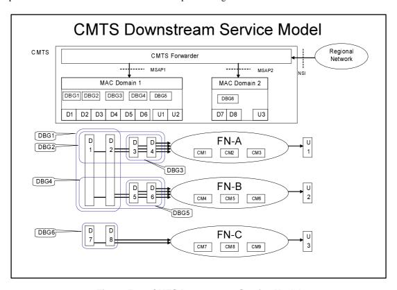
Figure 5-11: CMTS Downstream Service Model
