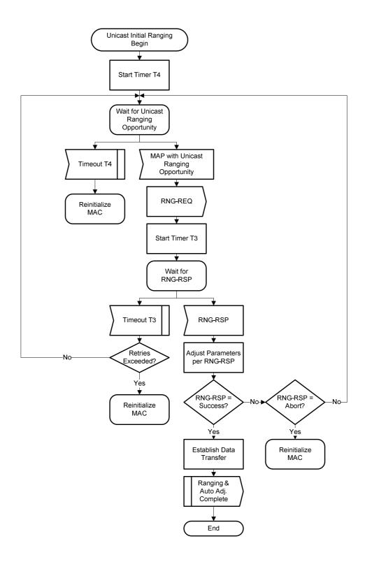
Figure 10-13: Unicast Initial Ranging - CM
