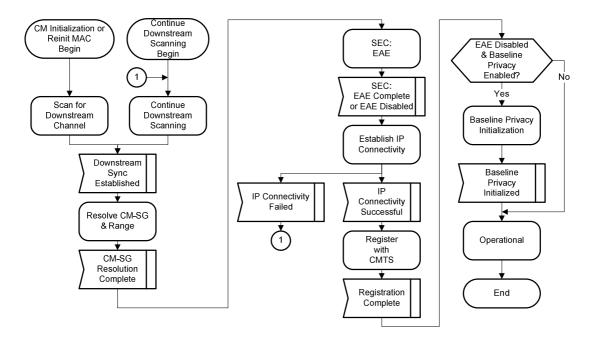
Figure 10-1: Cable Modem Initialization Overview
