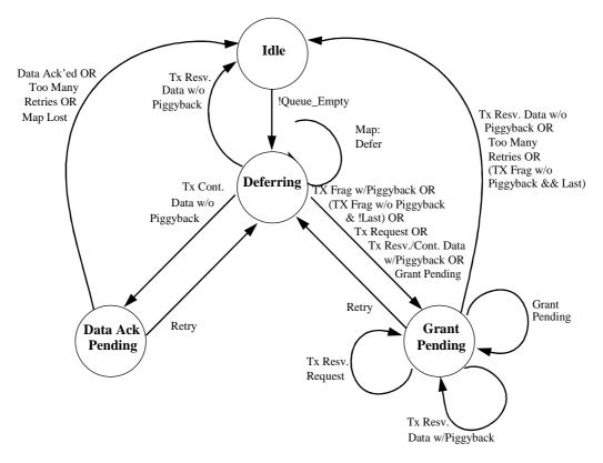
Figure N-2: Transmission and Deference State Transition Diagram
