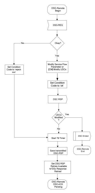
Figure 11-28: DSC-Remotely Initiated Transaction Begin State Flow Diagram
