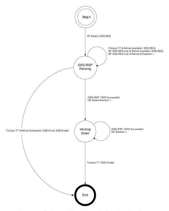
Figure 11-7: DSD-Locally Initiated Transaction State Transition Diagram
