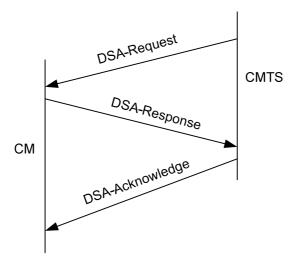
Figure 7-16: Dynamic Service Addition Message Flow - CMTS Initiated
