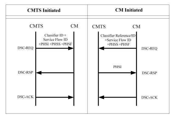
Figure 7-20: PHSI-Indexed Payload Header Suppression Signalling Example
