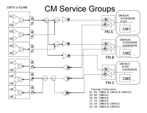
Figure 5-5: CM Topology Configuration Example
