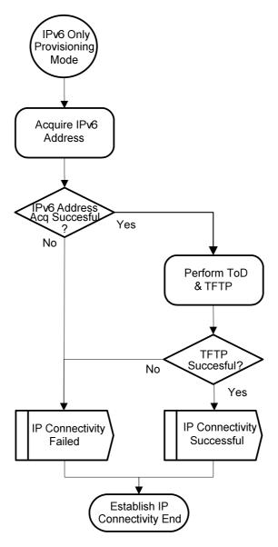
Figure 10-18: IPv6 Only Provisioning Mode
