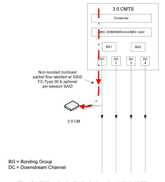
Figure S-1: Multicast Session Replication for a client behind a 2.0 CM
