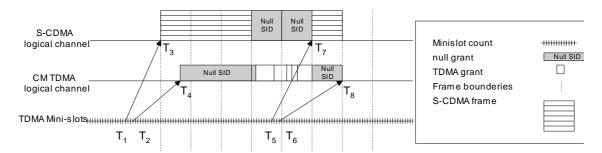
Figure 7-3: Logical S-CDMA TDMA channels
