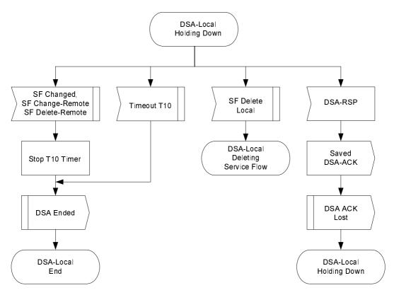
Figure 11-13: DSA-Locally Initiated Transaction Holding State Flow Diagram
