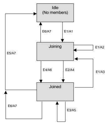
Figure T-1: IGMP Support - CM passive mode
