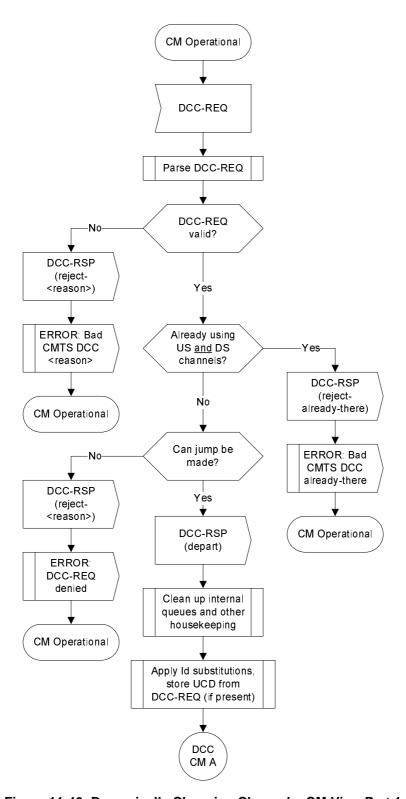
Figure 11-46: Dynamically Changing Channels: CM View Part 1
