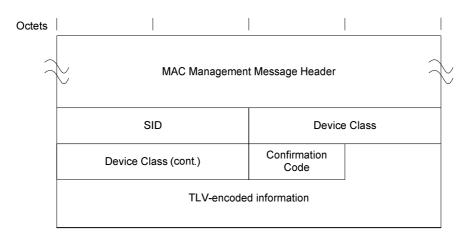
Figure 6-45: Device Class Identification Response
