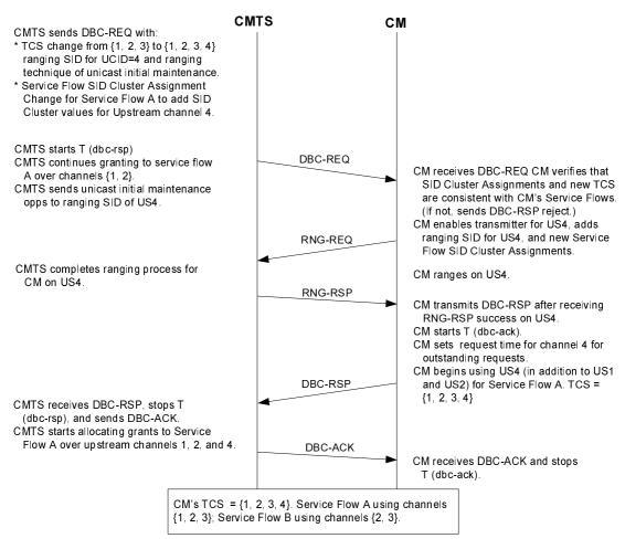
Figure W-2: Adding a Channel to the TCS and making a Service Flow SID Cluster Assignment
