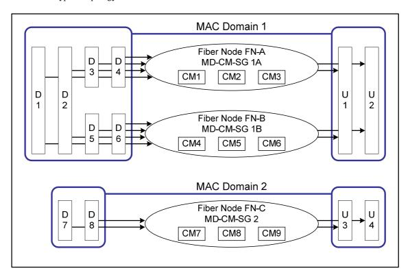
Figure 5-8: Example MAC Domain Channel Assignment
