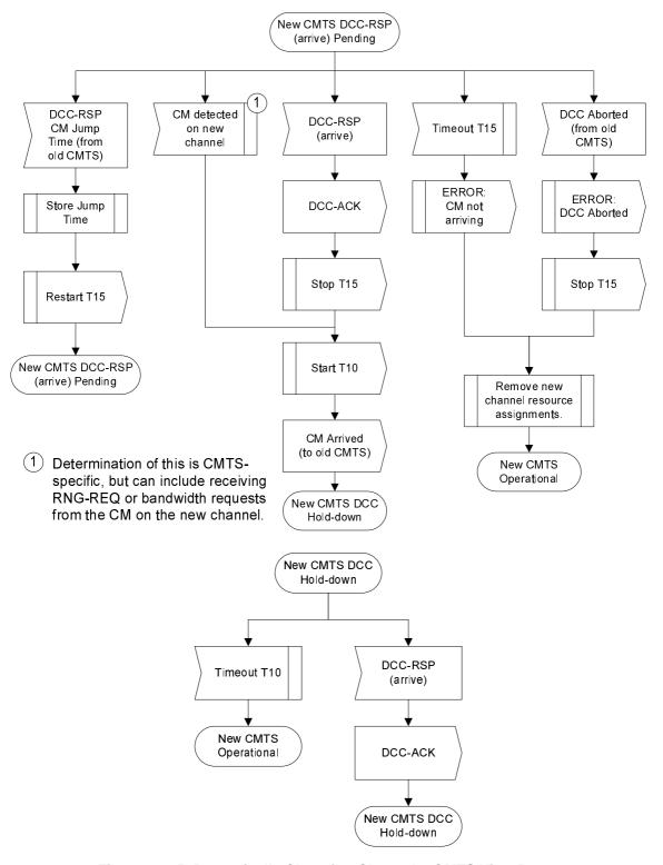
Figure 11-45: Dynamically Changing Channels: CMTS View Part 4
