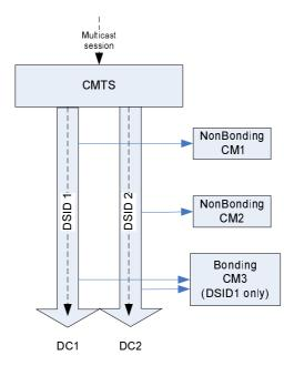
Figure 9-3: DSIDs prevent duplication of non-bonded replications
