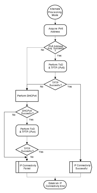
Figure 10-19: Alternate Provisioning Mode
