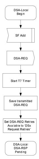
Figure 11-11: DSA-Locally Initiated Transaction Begin State Flow Diagram
