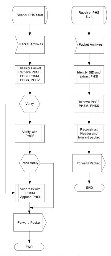
Figure 7-18: Payload Header Suppression Operation
