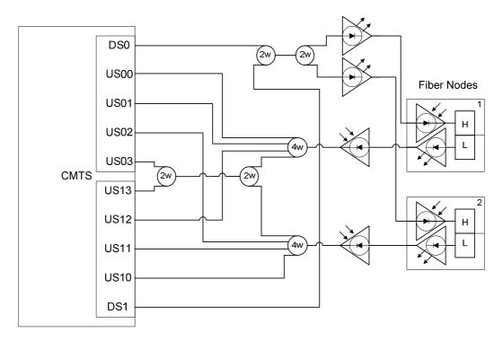
Figure W-5: Example Combining Network 2
