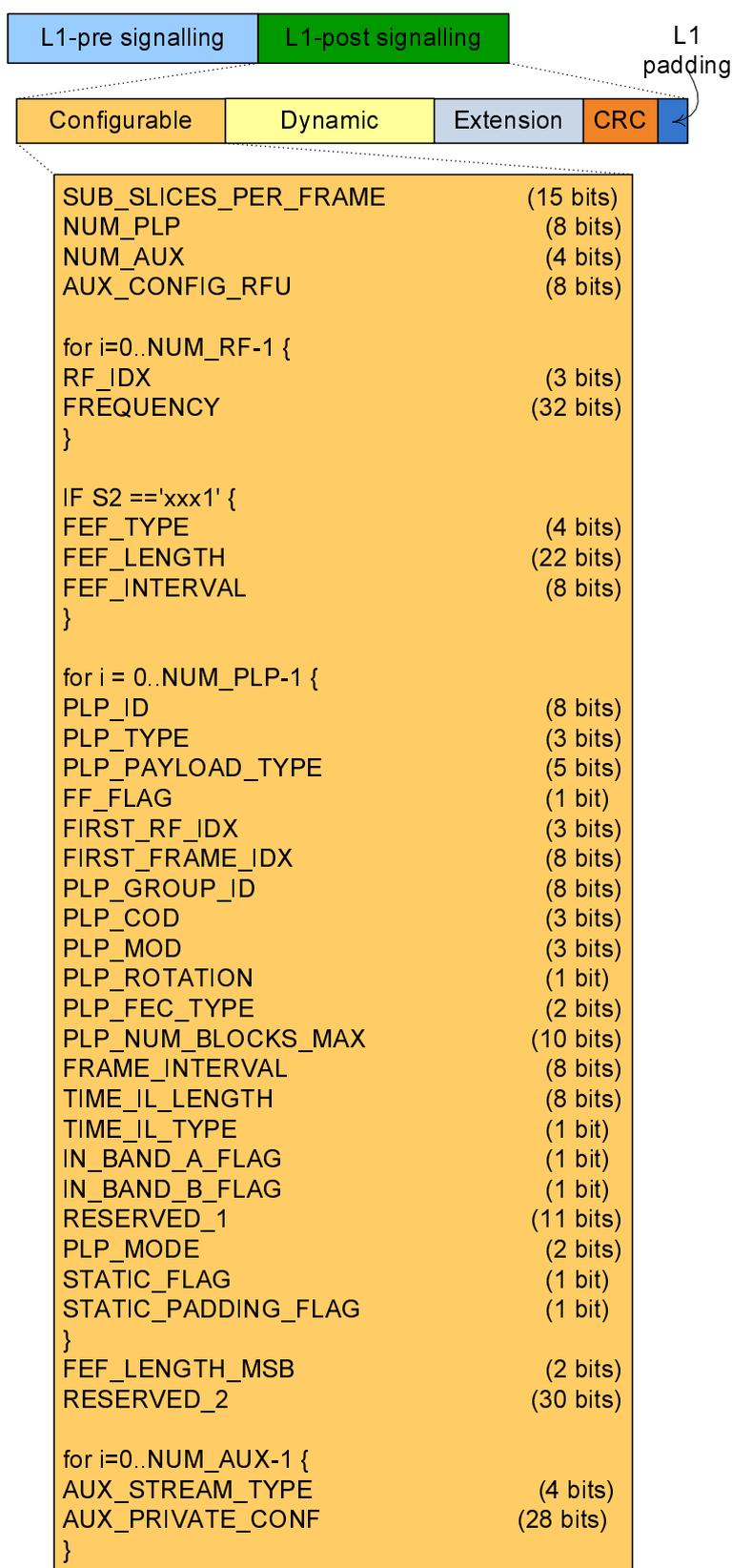
Figure 27: The signalling fields of configurable L1-post signalling
