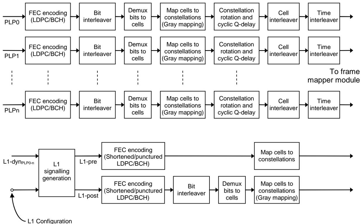
Figure 2(d): Bit Interleaved Coding and Modulation (BICM)
