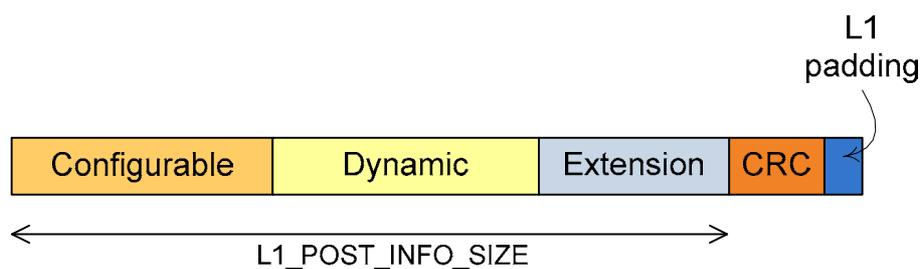
**Figure 26: The size indicated by the L1\_POST\_INFO\_SIZE field**
