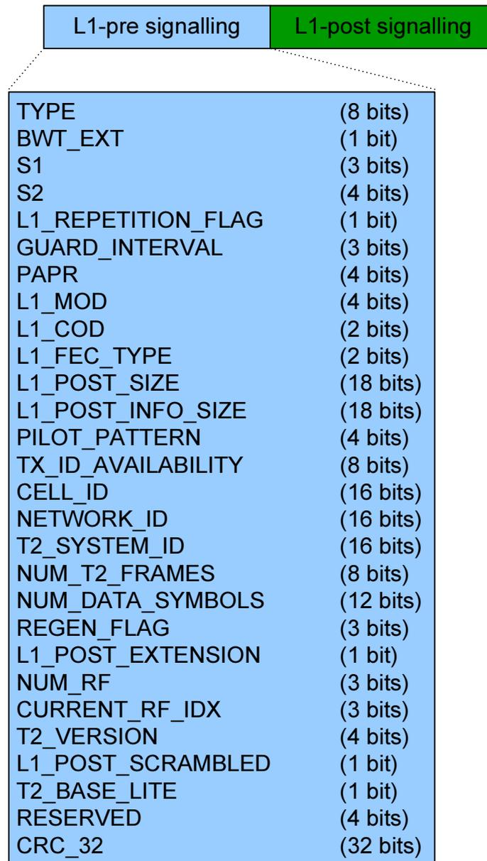
Figure 25: The signalling fields of L1-pre signalling
