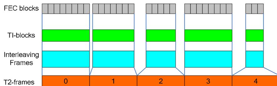
Figure 18(a): Time interleaving for  $P_1=1$ ,  $I_{JUMP}=1$ ,  $N_{TI}=1$
