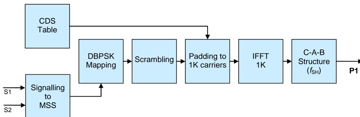
Figure 53: Block diagram of the P1 symbol generation
