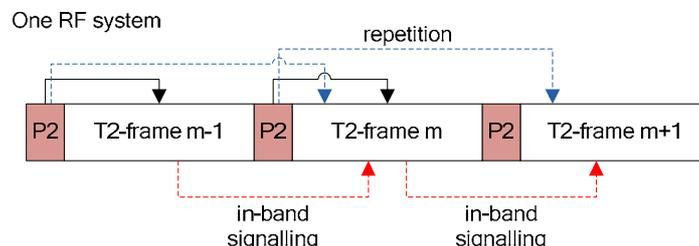
Figure 38: L1 signalling for a single RF system
