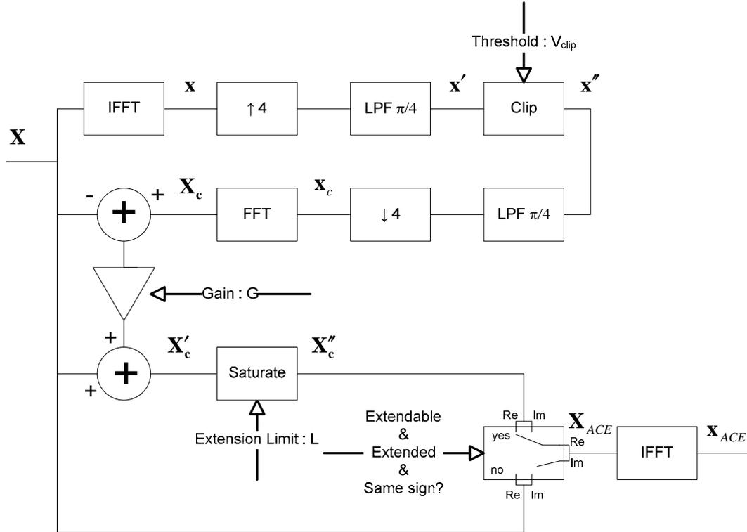
**Figure 50: Implementation of the Active Constellation Extension algorithm**
