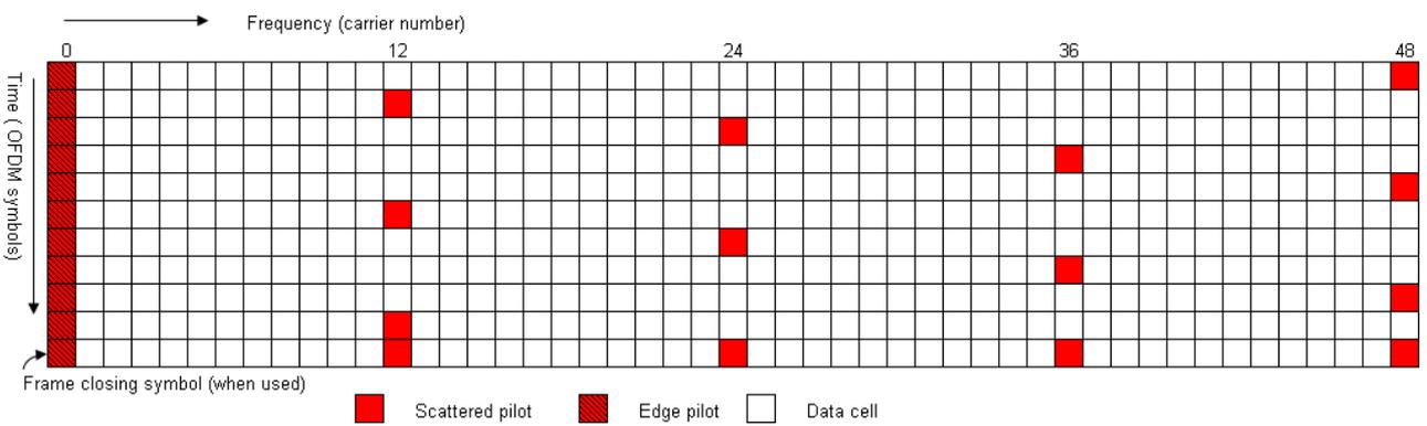
**Figure K.5: Scattered pilot pattern PP5 (SISO)**
