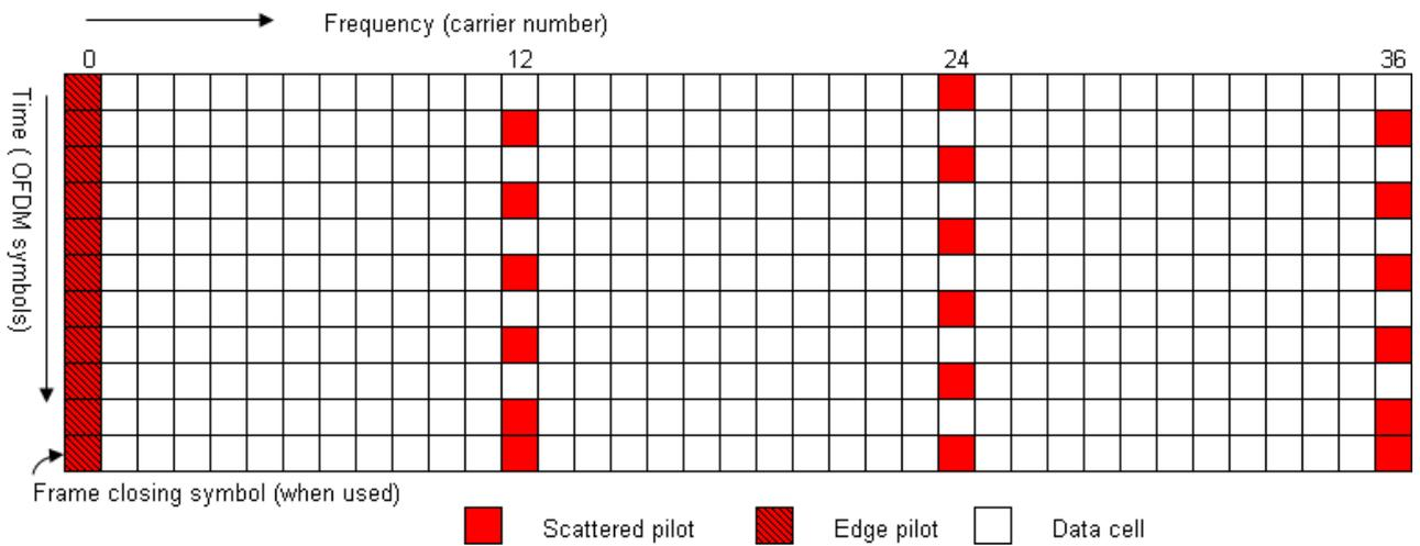
**Figure K.4: Scattered pilot pattern PP4 (SISO)**
