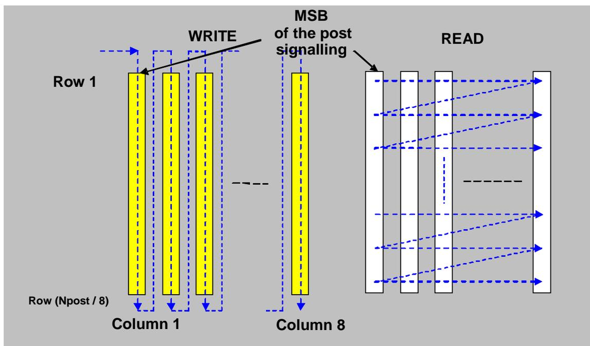
**Figure 34: Bit Interleaving scheme for L1-post (16-QAM)**
