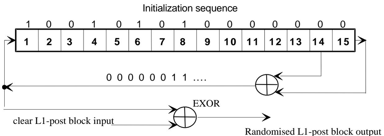
Figure 30: Possible implementation of the PRBS encoder
