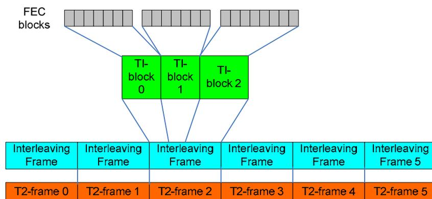
Figure 18(c): Time interleaving for  $P_1=1$ ,  $I_{JUMP}=1$ ,  $N_{TI}=3$
