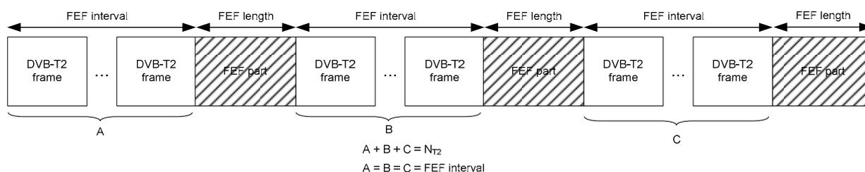
**Figure 36: The super-frame, including T2-frames and FEF parts**
