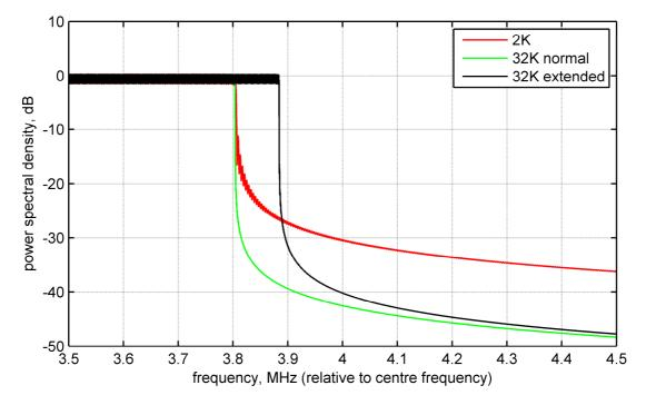
Figure 52(b): Detail of theoretical DVB-T2 spectrum for guard interval fraction 1/8 (for 8 MHz channels)
