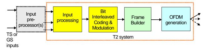
Figure 1: High level T2 block diagram
