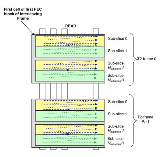
Figure 22: The output from a single TI-block, split into  $N_{\text{subslices}}$  sub-slices in each of  $P_{\text{I}}$  T2-frames
