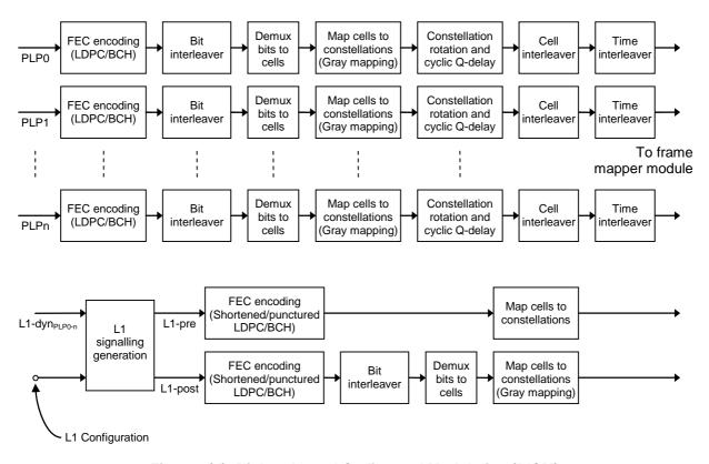
Figure 2(d): Bit Interleaved Coding and Modulation (BICM)
