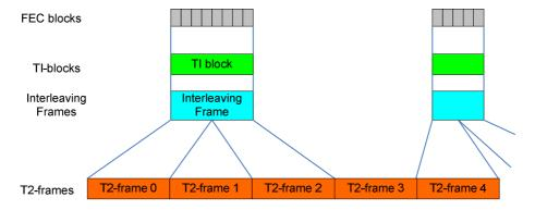
Figure 18(b): Time interleaving for  $P_i=2$ ,  $I_{HIMP}=2$ ,  $N_{Ti}=1$
