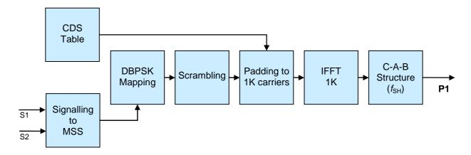
Figure 51: Block diagram of the P1 symbol generation
