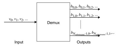
Figure 14: De-multiplexing of bits into sub-streams
