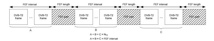
Figure 35: The super-frame, including T2-frames and FEF parts
