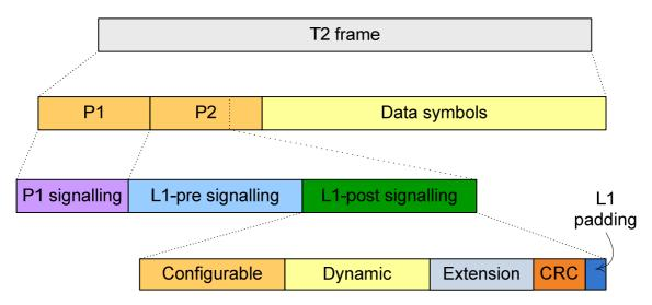
Figure 24: The L1 signalling structure
