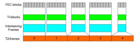
Figure 18(a): Time interleaving for  $P_{i}=1$ ,  $I_{JUMP}=1$ ,  $N_{Ti}=1$
