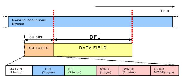
Figure 7: Stream format at the output of the MODE ADAPTER, Normal Mode (GSE & GCS)
