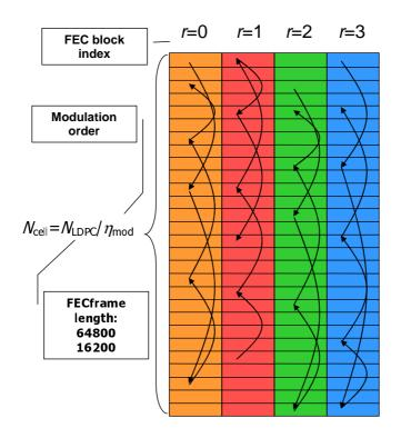
Figure 17: Cell Interleaving scheme
