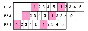
Figure E.3(a): The structure of the type 2 part of a T2-frame with  $N_{RF} = 3$  and  $N_{\text{subslices\_total}} = 6$  before folding, showing the sub-slices exceeding the frame
