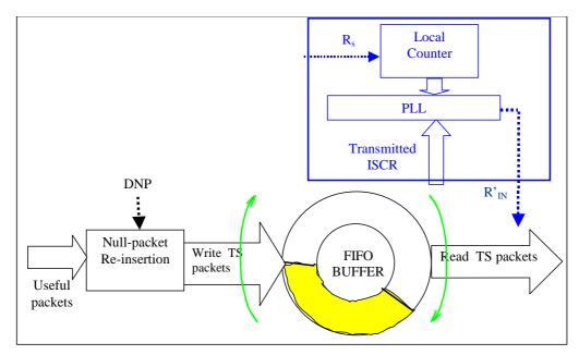
Figure I.1: Example receiver block diagram for Null-packet re-insertion and R<sub>TS</sub> clock recovery
