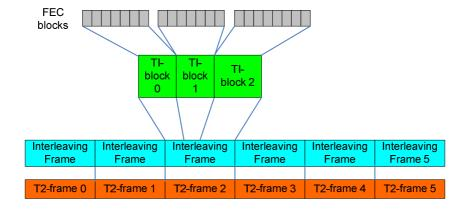
Figure 18(c): Time interleaving for  $P_{i=1}$ ,  $I_{JUMP}=1$ ,  $N_{Ti}=3$
