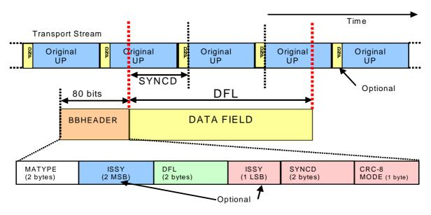
Figure 6: Stream format at the output of the MODE ADAPTER, High Efficiency Mode for TS, (no CRC-8 computed for UPs, optional single ISSY inserted in the BBHEADER, UPL not transmitted)
