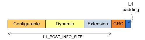
Figure 26: The size indicated by the L1\_POST\_INFO\_SIZE field
