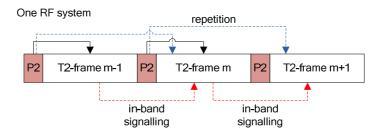
Figure 37: L1 signalling for a single RF system
