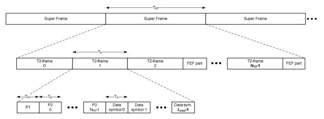
Figure 34: The DVB-T2 frame structure, showing the division into super-frames, T2-frames and OFDM symbols
