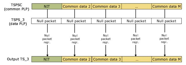
Figure D.2: Example of recombination of input TS from TSPS and TSPSC for category 1
