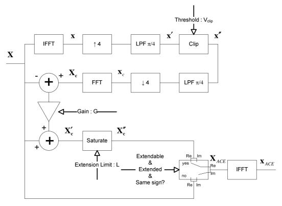
Figure 48: Implementation of the Active Constellation Extension algorithm
