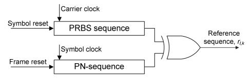
Figure 46: Formation of the reference sequence from the PN and PRBS sequences
