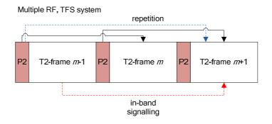
Figure E.6: L1 signalling for a TFS system
