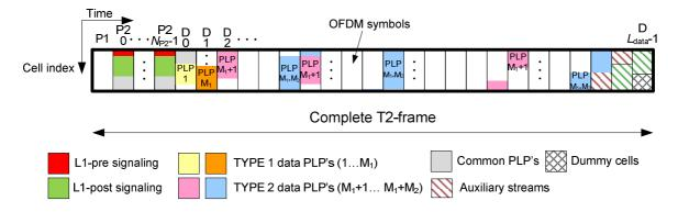
Figure 38: Mapping of data PLPs into the data symbols
