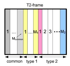
Figure 41: Allocation of  $M_{\text{common}}$  common PLPs,  $M_1$  data PLPs of type1 and  $M_2$  data PLPs of type 2 transmitted in one T2-frame
