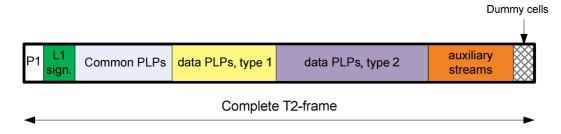
Figure 36: Structure of the T2-frame
