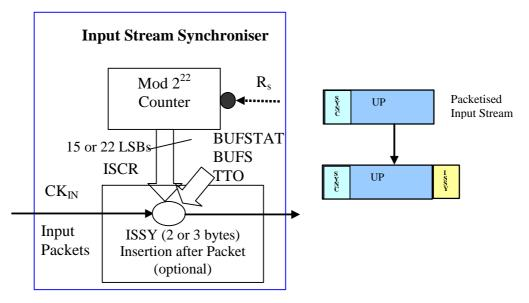
Figure C.1: Input stream synchronizer block diagram
