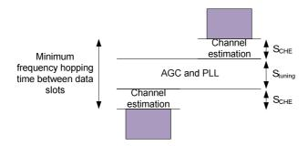
Figure E.5: Minimum required frequency hopping time between two sub-slices to be received with the same tuner
