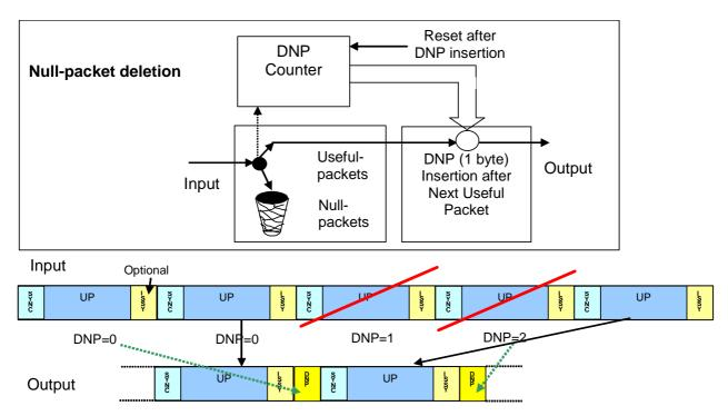
Figure 3: Null packet deletion scheme
