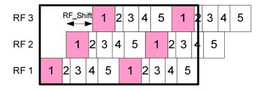
Figure E.8: Cell allocations for the sub-slices prior to "folding"
