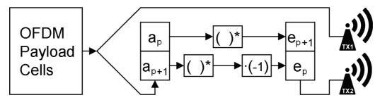
Figure 45: Multiple Input, Single Output, Encoder processing of OFDM payload cells
