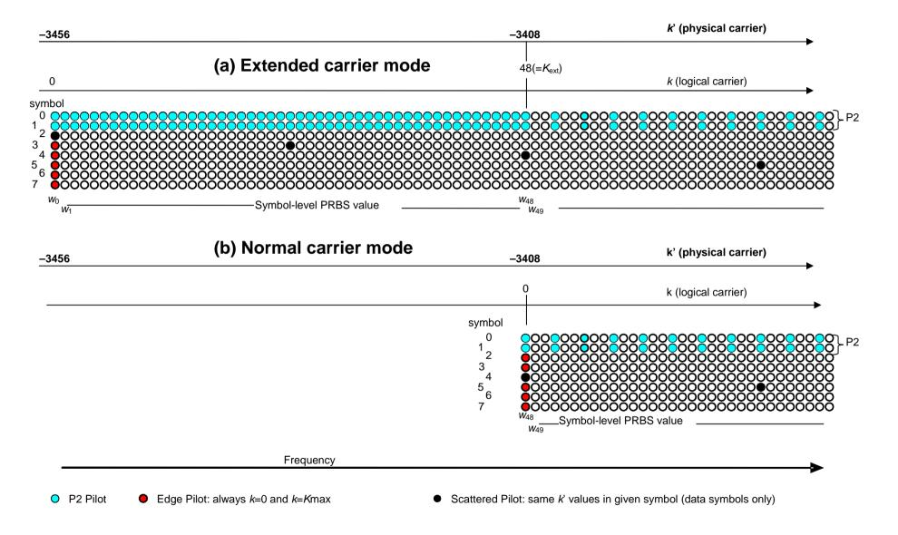
Figure J.17: Example of pilot and TR cells at the edge of the spectrum in extended and normal carrier mode (8K PP7)
