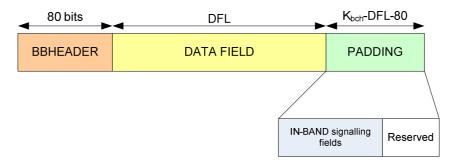
Figure 10: PADDING format at the output of the STREAM ADAPTER for in-band type A
