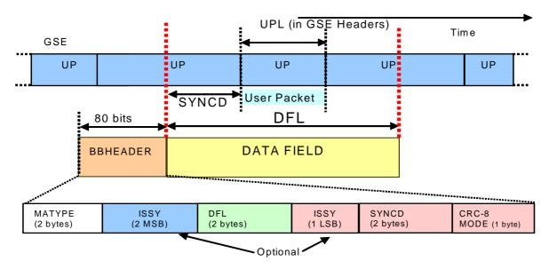
Figure 8: Stream format at the output of the MODE ADAPTER, High Efficiency Mode for GSE, (no CRC-8 computed for UPs, optional single ISSY inserted in the BBHEADER, UPL not transmitted)
