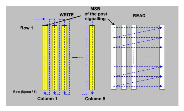
Figure 33: Bit Interleaving scheme for L1-post (16-QAM)
