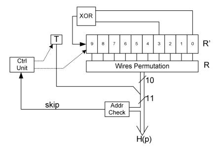
Figure 44(b): Frequency interleaver address generation scheme for the 2k mode
