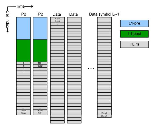
Figure 42: Addressing of the OFDM cells for common PLPs and data PLPs
