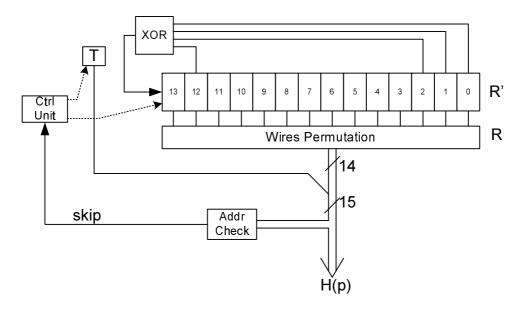
Figure 44(f): Frequency interleaver address generation scheme for the 32k mode
