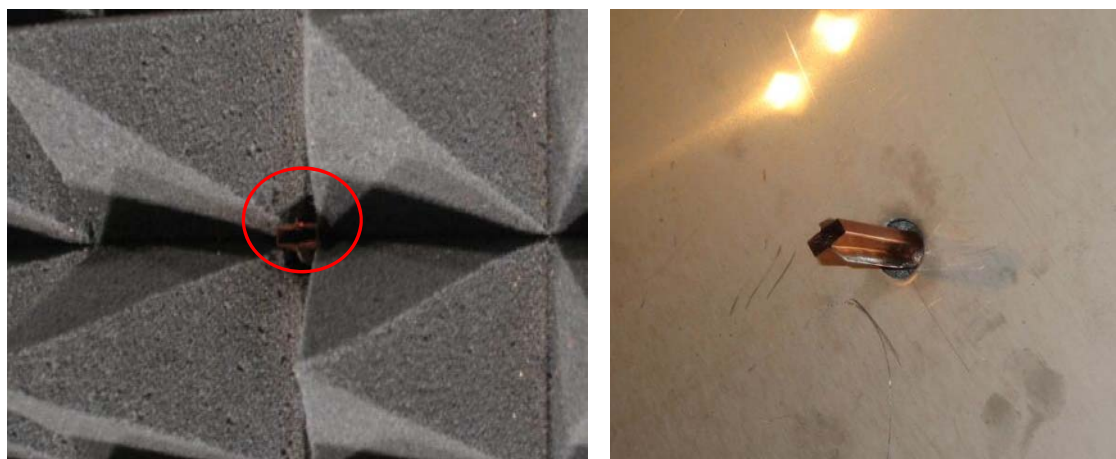
Figure 7: Left: Horn antenna fitted in pyramidal absorbers; Right: Horn antenna protruding the centre of the metal plate
