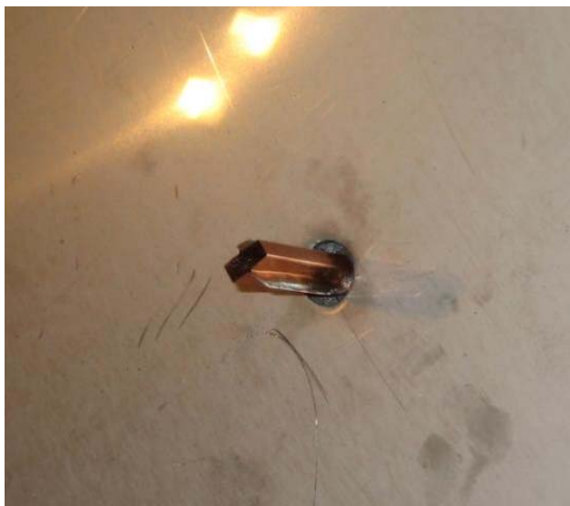
Figure 7: APC measurement setup - Details of open ended waveguide trough the metal
