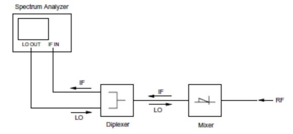
Figure J.1: Set-up of measurement receiver, diplexer and mixer
