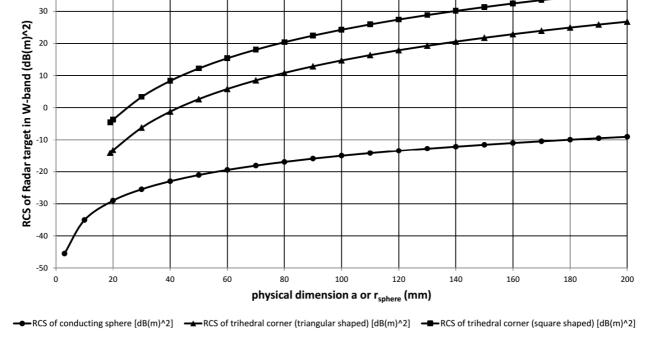
Figure K.5: Radar cross sections as a function of the physical dimensions of different targets for W-band frequencies (wavelength 3,75 mm)
