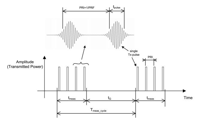
Figure H.1: Typical pulse modulation scheme
