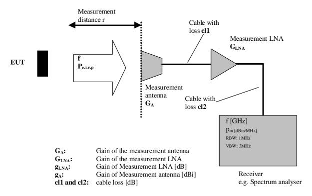
Figure 2: Test set-up for measuring the operating bandwidth
