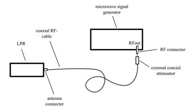
Figure 7: Conducted test setup for the alternative scenario
