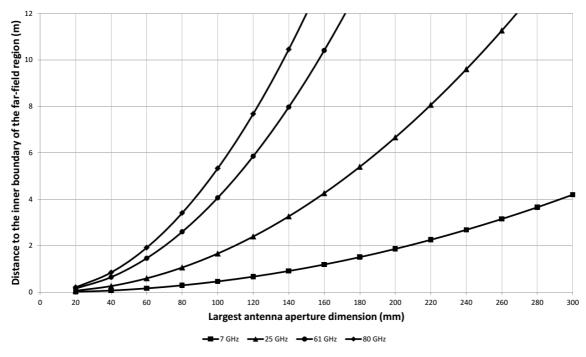
Figure L.1: Correlation between far-field distance and antenna aperture dimension for the different LPR frequency bands
