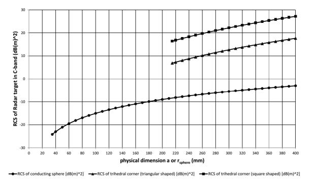
Figure K.2: Radar cross sections as a function of the physical dimensions of different targets for C-band frequencies (wavelength 42,8 mm)
