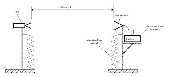
Figure 6: Radiated test setup for the alternative scenario
