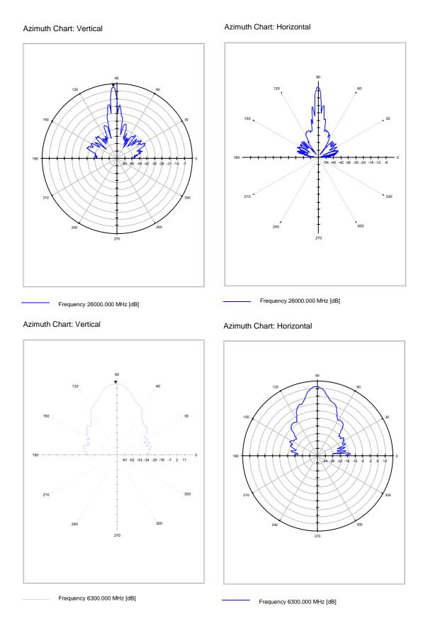
Figure 8: Examples of LPR antenna characteristics
