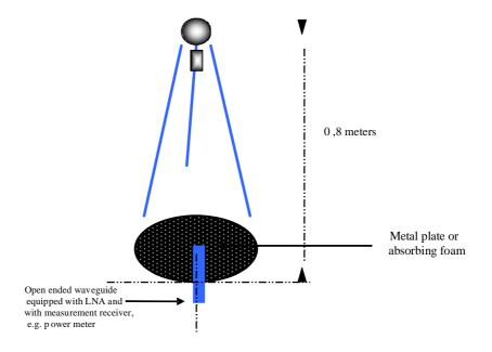
Figure 9: APC measurement setup
