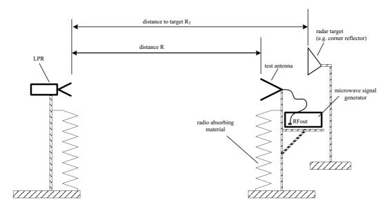
Figure 3: Radiated test setup for the equivalent scenario
