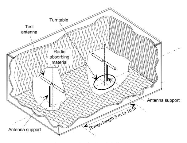
Figure C.1: A typical Anechoic Chamber
