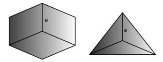
Figure K.1: Different corner reflectors (left hand side: square shaped, right hand side: triangular shaped)
