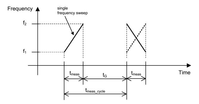
Figure H.2: Typical FMCW modulation scheme
