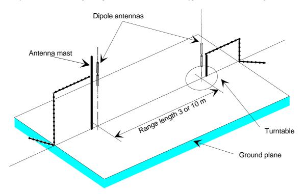
Figure C.3: A typical Open Area Test Site
