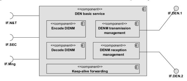
Figure 3: DEN basic service component diagram
