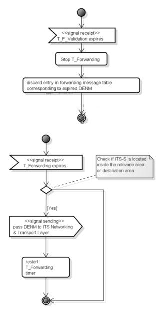
Figure 12: Forwarding ITS-S activity diagram: timeout management
