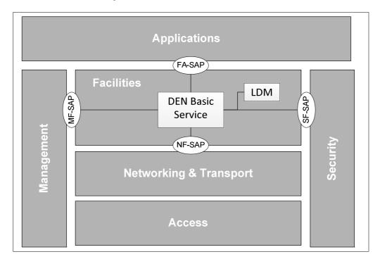
Figure 2: DEN basic service and logical interfaces
