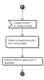
Figure 14: Receiving ITS-S activity diagram: timeout management
