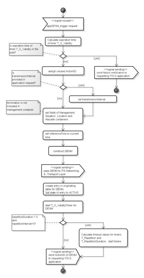
Figure 7: Originating ITS-S activity diagram: appDENM\_trigger request
