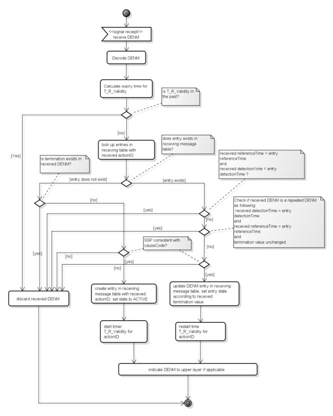
Figure 13: Receiving ITS-S activity diagram
