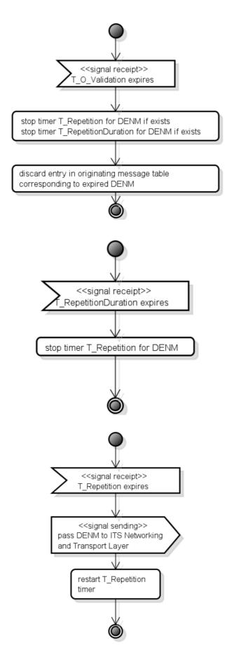
Figure 10: Originating ITS-S activity diagram: timeout management
