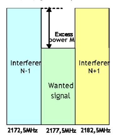
Figure 1: Adjacent channel spectrum
