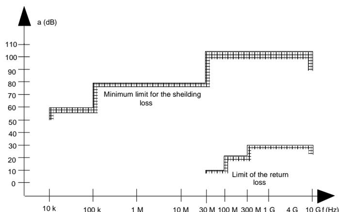
Figure B.2: Specification for shielding and reflections
