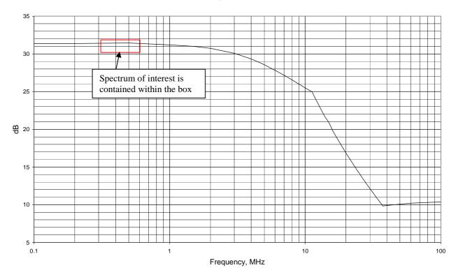
Figure D.2: Conversion factor C<sub>3</sub> versus frequency
