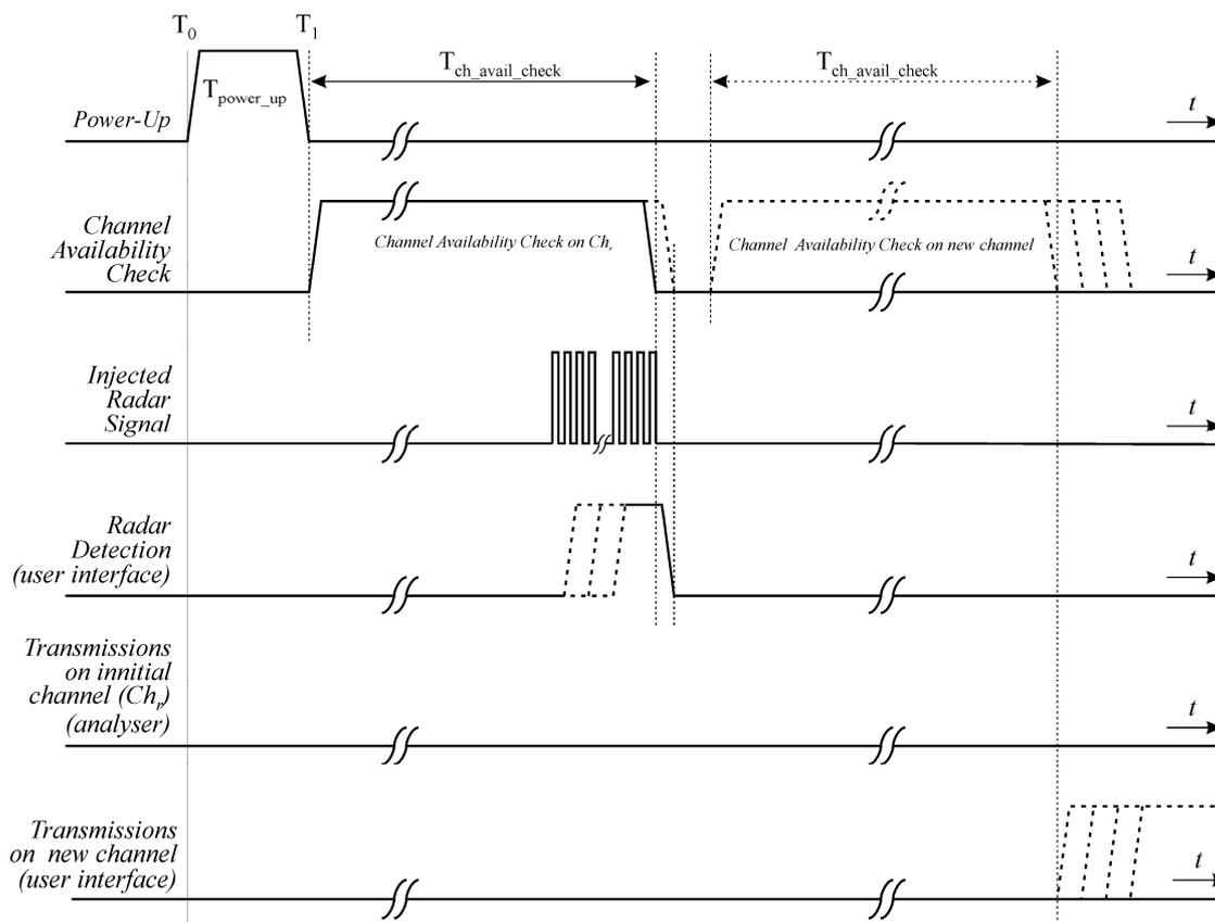
**Figure 5: Example of timing for radar testing towards the end of the Channel Availability Check Time**
