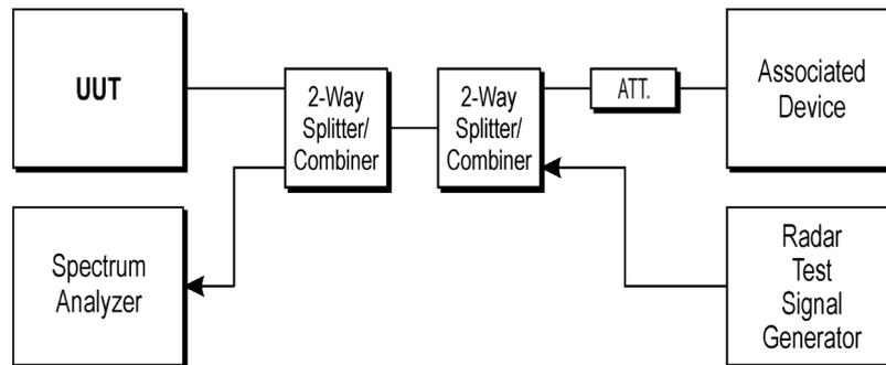
NOTE: UUT can be any type of FWA Device under test. An Associated Device is the equipment required for the UUT to establish a communication link.
