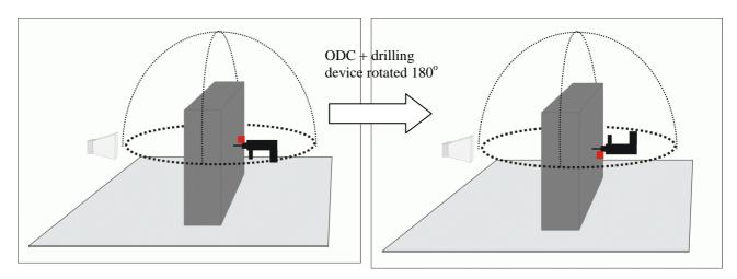
Figure 6: Measurement arrangement for all emission measurements (TE, UE, OE, UE-TP) for Category B equipment
