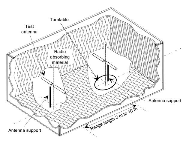
Figure A.1: A typical anechoic chamber
