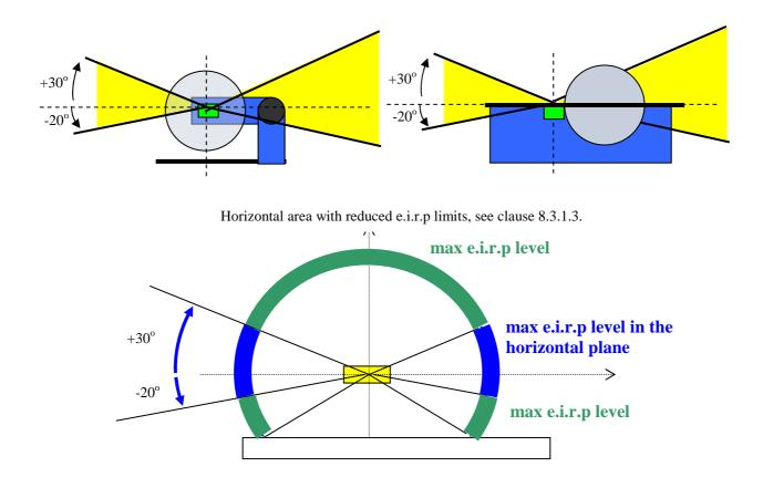
Figure 7b: Spatial requirements for the test set-up
