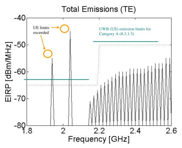
Figure 3: Example for a TE measurement in the frequency range 1,8 GHz to 2,6 GHz
