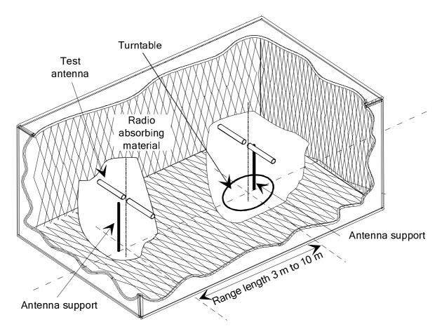
Figure A.1: A typical anechoic chamber
