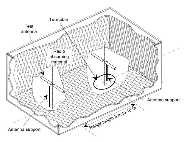
Figure A.1: A typical anechoic chamber
