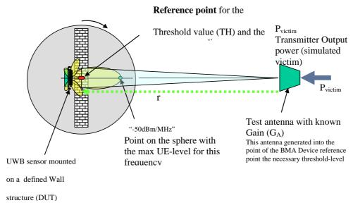
Figure 6: Test set-up for LBT function
