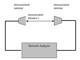
Figure D.1: Calibration setup
