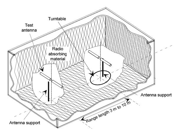
Figure A.1: A typical Anechoic Chamber
