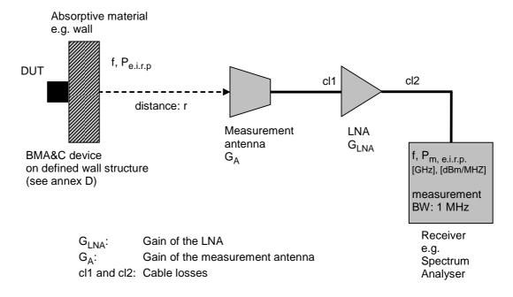
Figure 1: Test set-up for measuring the operating frequency range
