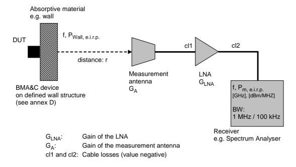
Figure 3: Test set-up for e.i.r.p measurements
