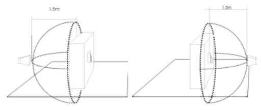
Figure 2: Measurement arrangement for all emission measurements (TUE, USE, UE, UE-TP)
