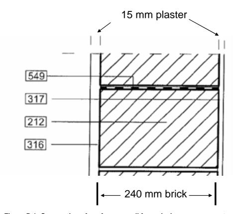
Figure D.1: Crossection of a reference wall for emission measurements
