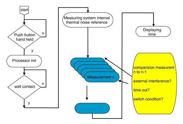
Figure 5: Flow diagram of LBT mechanism
