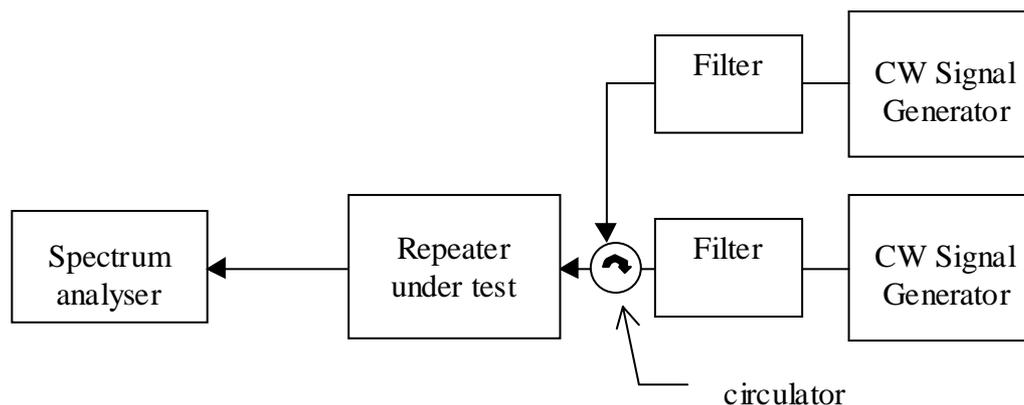
Figure D.3: Measuring system set-up for input intermodulation
