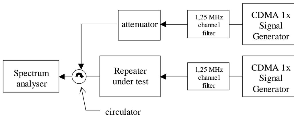
Figure D.6: Measuring system set-up for output intermodulation
