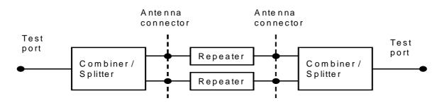
Figure B.1: Example of repeater configuration
