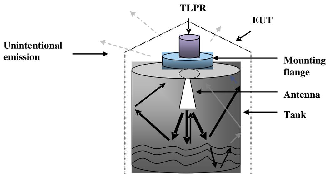
Figure D.1: A typical unintentional emission pattern from the EUT
