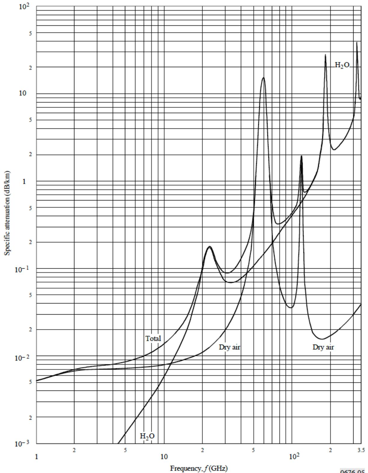
Figure H.1: Specific attenuation due to atmospheric gases in the band 1 GHz to 350 GHz in dB/km
