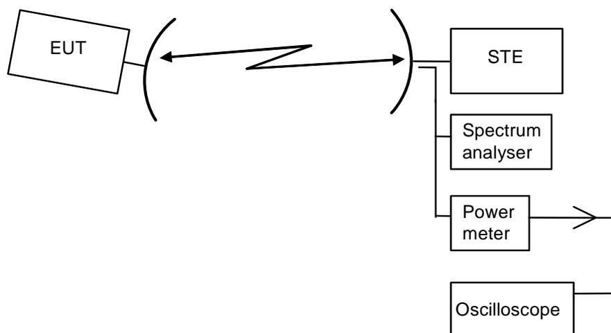
Figure 11: Test arrangement for pointing error detection
