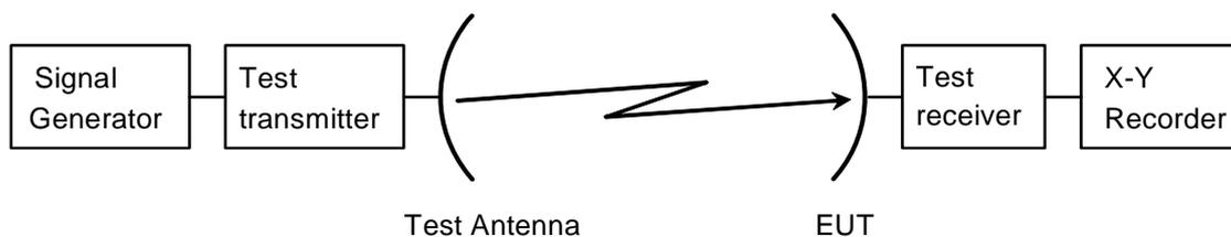
**Figure 10: Test arrangement - antenna transmit radiation pattern measurement**
