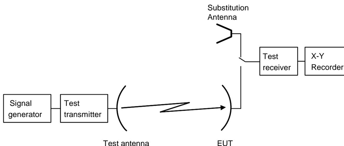
**Figure 9: Test arrangement - antenna transmit gain measurement**
