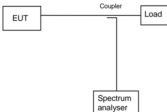
**Figure 8: Test arrangement - transmit output power density measurement**
