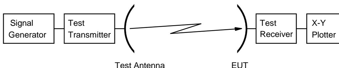
**Figure 14: Test arrangement - antenna receive pattern measurement**
