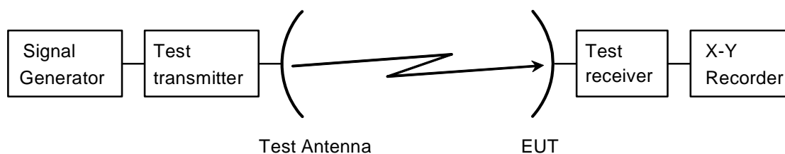
Figure 10: Test arrangement - antenna transmit radiation pattern measurement
