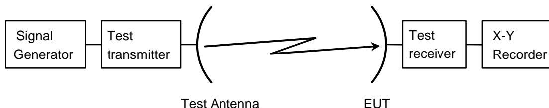
Figure 10: Test arrangement - antenna transmit radiation pattern measurement
