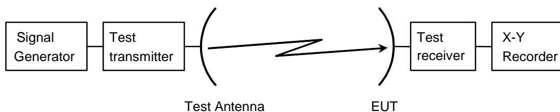
Figure 10: Test arrangement - antenna transmit radiation pattern measurement
