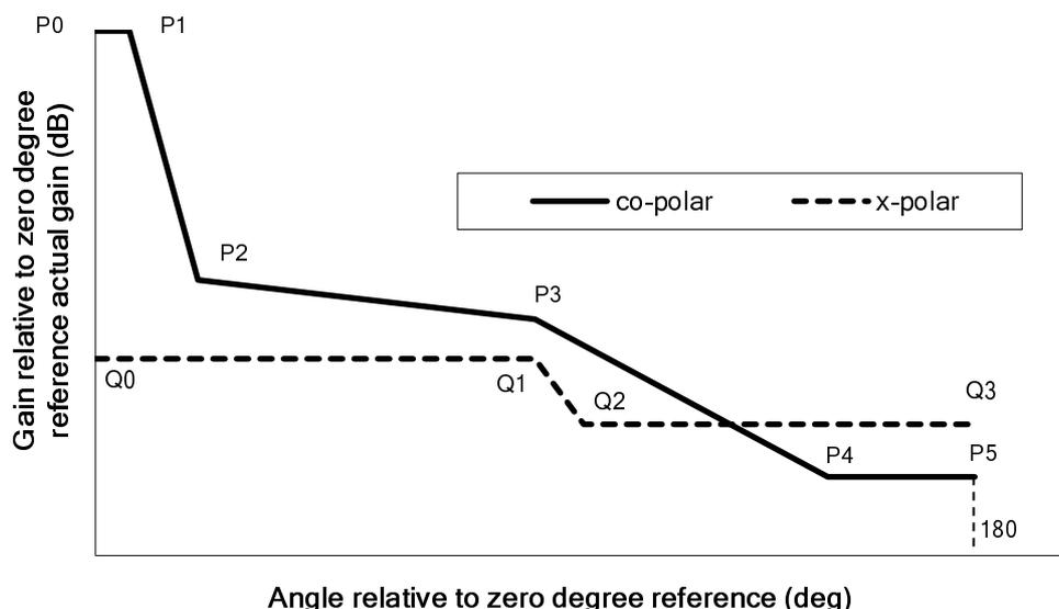
**Figure 3: Normalized RPE for DN Azimuth and Elevation**
