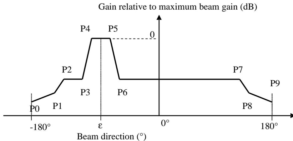
**Figure 8: Azimuth RPEs for linear polarized multi-beam sector antennas 3 GHz to 5,9 GHz (defined for each beam)**
