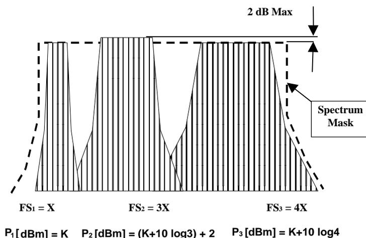
**Figure 5: Example of equipment with EqC-PET = M, with three sub-carriers, each with a different Symbol Frequency (SF)**
