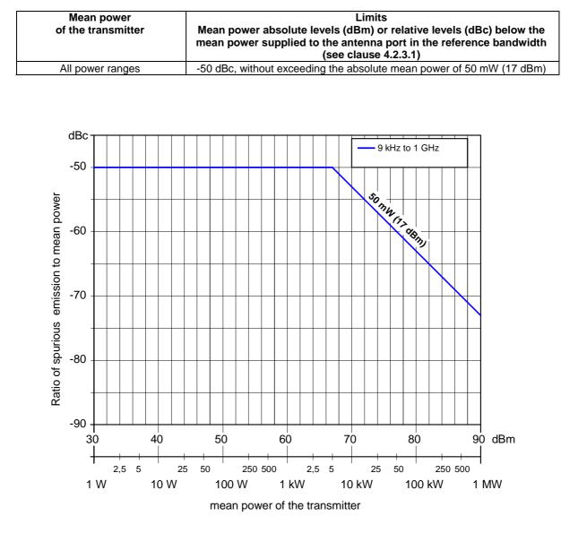
Table 1: Spurious emission limits for DRM transmitters operating below 30 MHz
