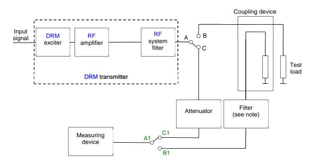
For high power transmitters the preferred set up requires A to be connected to B and A1 to be connected to B1. For low power transmitters the preferred set up requires A to be connected to C and A1 to be connected to C1.
