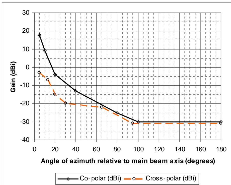
Figure 13: Class 4 antennas RPE (14 GHz to 20 GHz)
