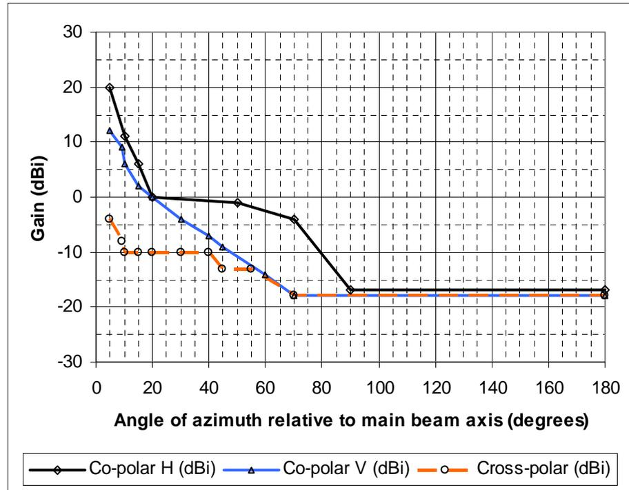
Figure 23: Class 3C antennas RPE (30 GHz to 47 GHz)
