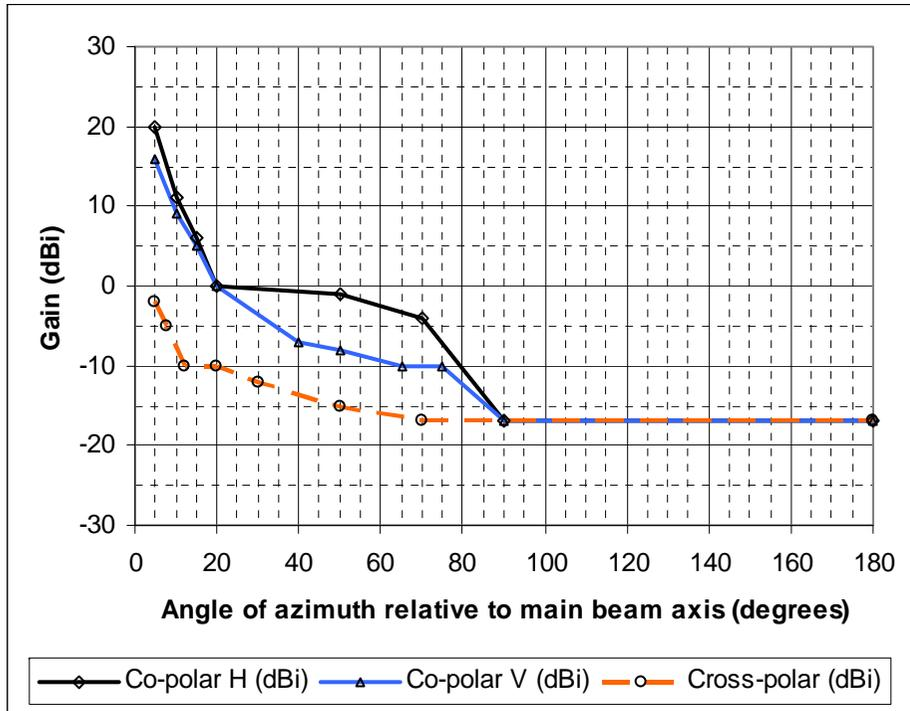
Figure 22: Class 3B antennas RPE (30 GHz to 47 GHz)
