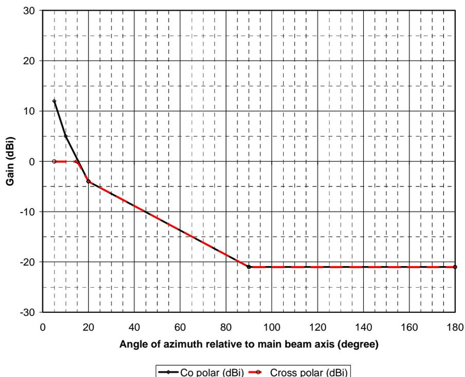
Figure 30: Class 4 antenna RPE (71 GHz to 86 GHz)
