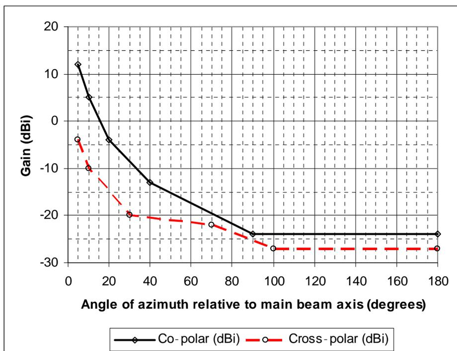
Figure 24: Class 4 antennas RPE (30 GHz to 47 GHz)
