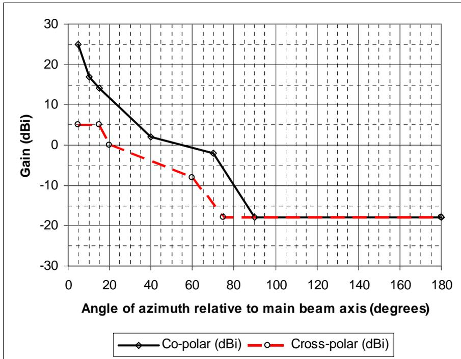
Figure 25: Class 2 antennas RPE (47 GHz to 66 GHz)
