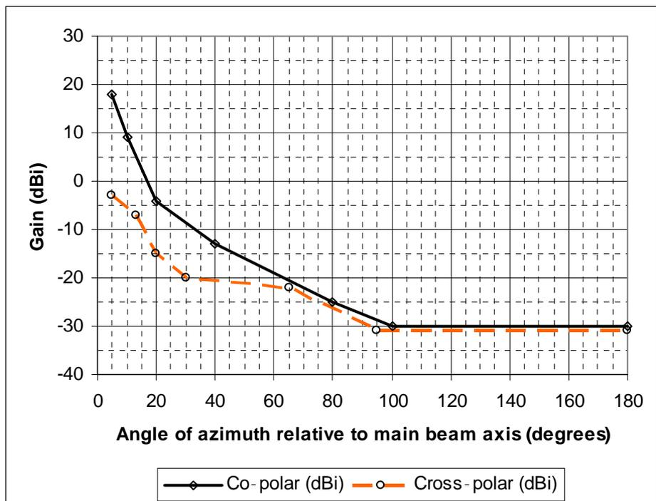
Figure 19: Class 4 antennas RPE (24 GHz to 30 GHz)
