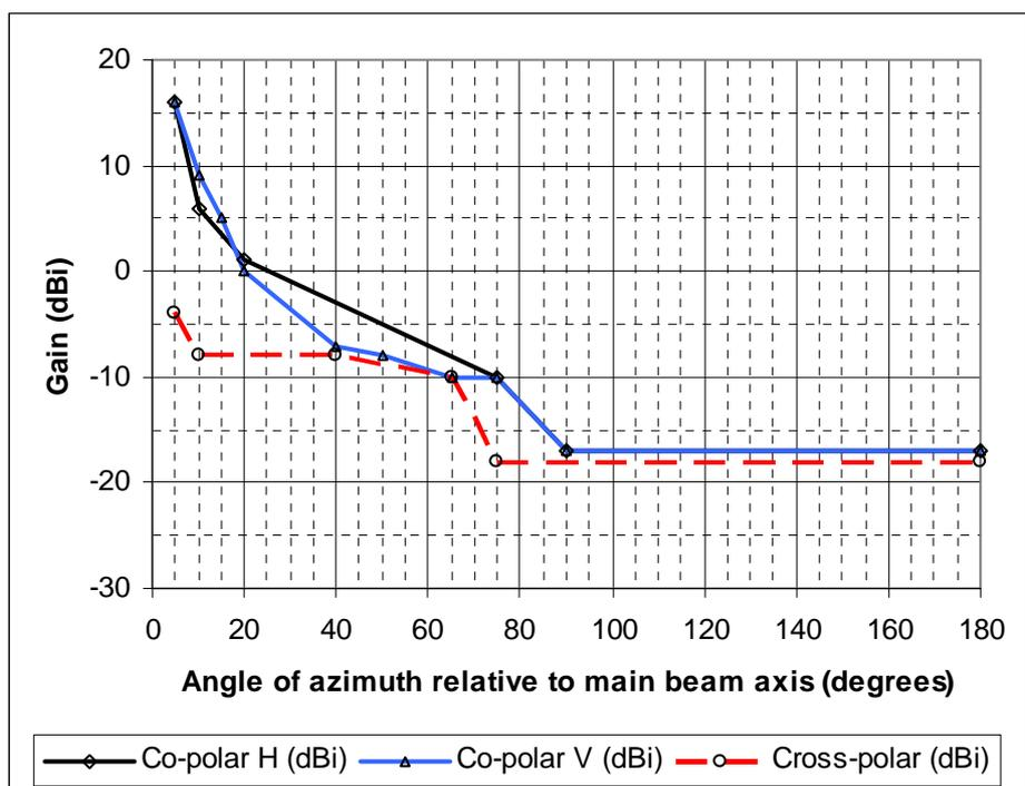
Figure 27: Class 3B antennas RPE (47 GHz to 66 GHz range)
