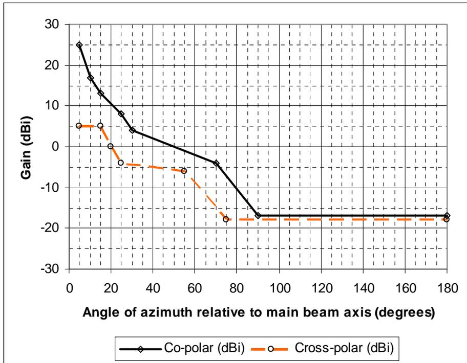
Figure 20: Class 2 antennas RPE (30 GHz to 47 GHz)
