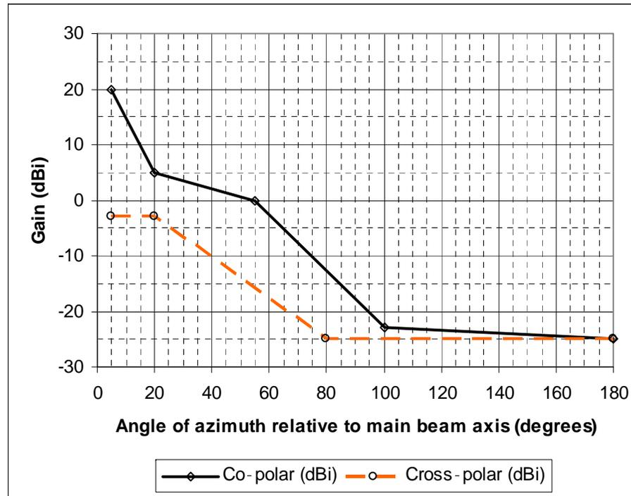
Figure 18: Class 3 antennas RPE (24 GHz to 30 GHz)
