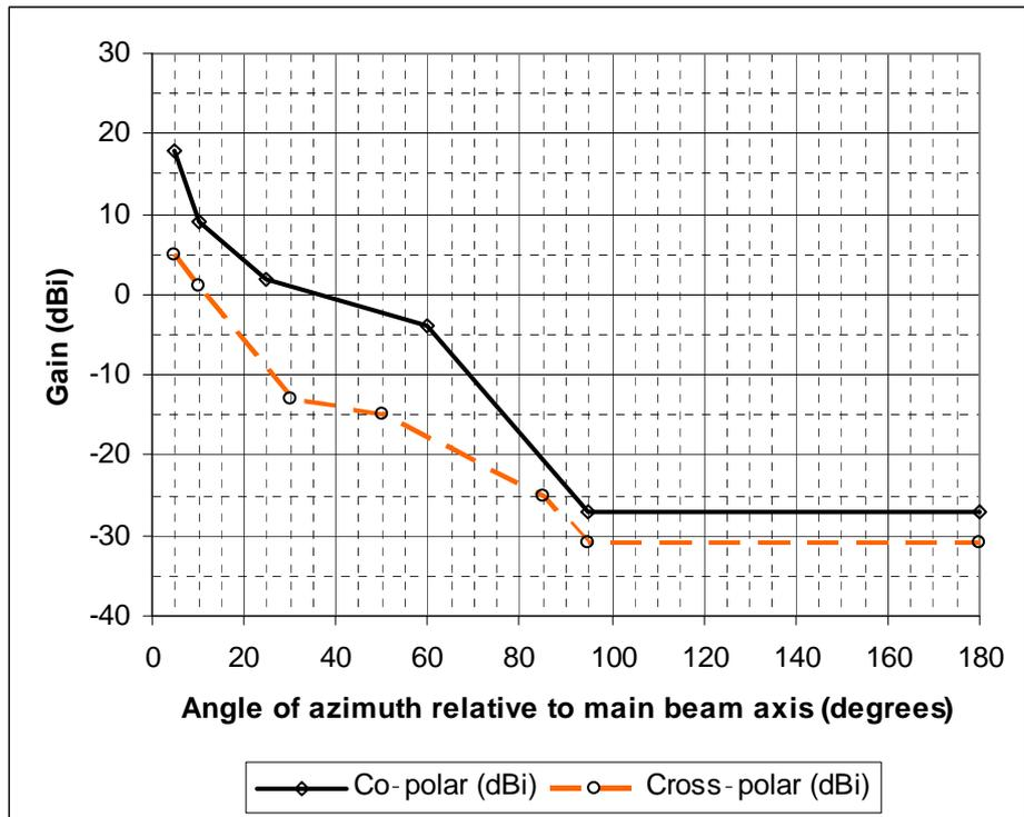
Figure 12: Class 3 antennas RPE (14 GHz to 20 GHz)
