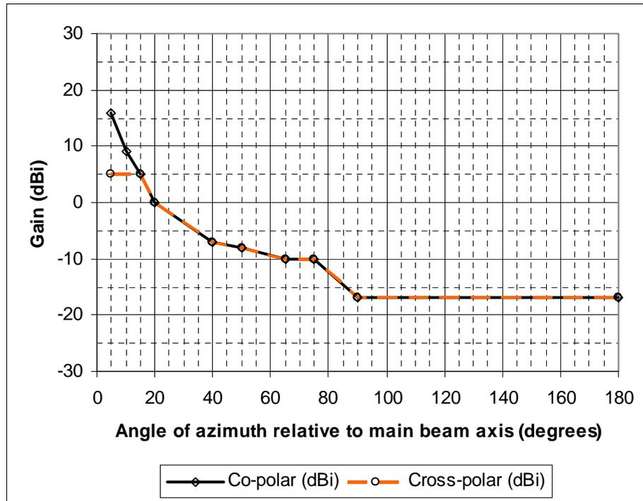
Figure 21: Class 3 A antennas RPE (30 GHz to 47 GHz, applicable to single vertical polarized antennas only)
