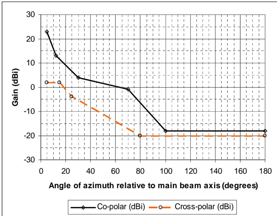
Figure 17: Class 2 antenna RPE (24 GHz to 30 GHz)
