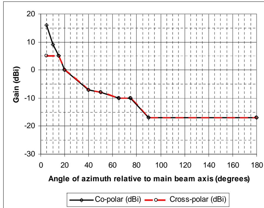
Figure 26: Class 3A antennas RPE (47 GHz to 66 GHz, vertically polarized only)
