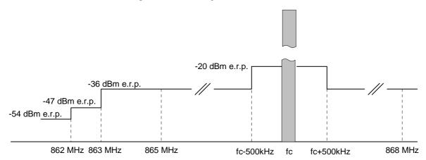
NOTE 1: fc is the centre frequency of the carrier transmitted by the interrogator.
