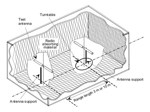
Figure A.1: A typical anechoic chamber
