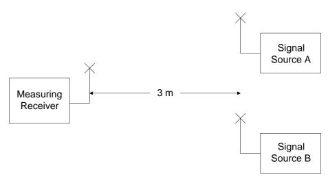
Figure B.3: Calibration of field levels
