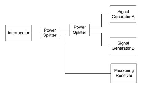
Figure B.5: Conducted measurement of blocking
