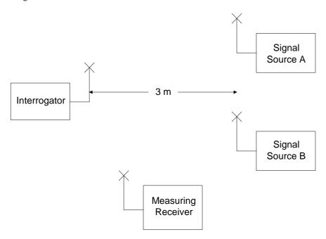
Figure B.4: Radiated measurement of blocking
