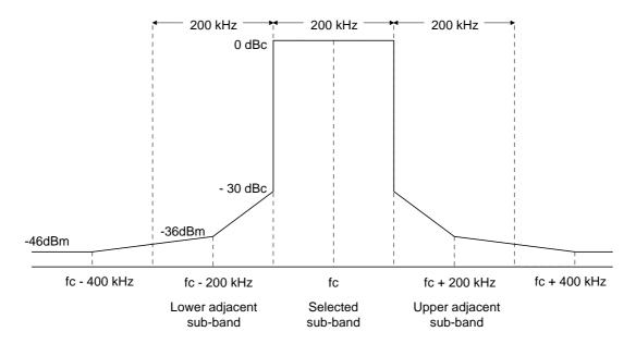
NOTE 1: Where fc is the centre frequency of the carrier transmitted by the interrogator.
