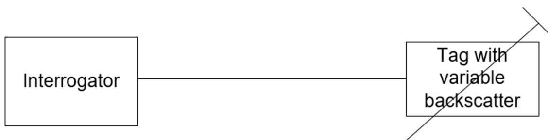
Figure 13: Conducted test set up for receiver sensitivity with (emulated) tag with variable backscatter
