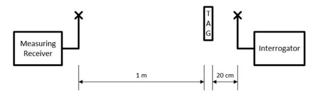
Figure 16: Measurement of tag emissions
