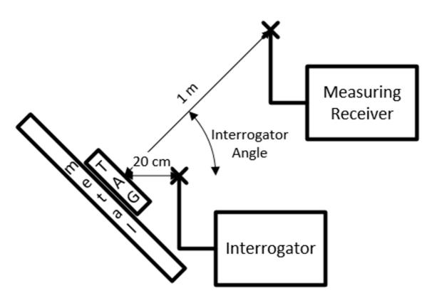
Figure 17: Measurement of tag emissions with metal
