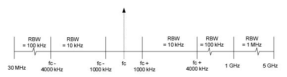
Figure 9: Resolution bandwidths for spurious emission in the upper band
