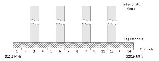
Figure 2: Channel plan for upper band
