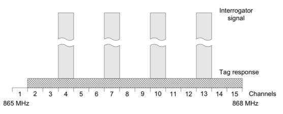
Figure 1: Channel plan for lower band
