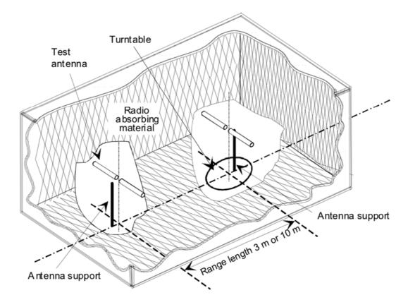
Figure B.1: A typical anechoic chamber
