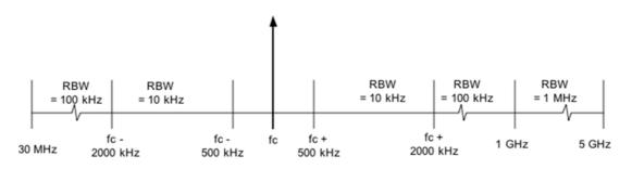
Figure 8: Resolution bandwidths for spurious emission in the lower band
