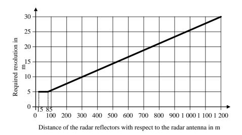
Figure B.4: Required Azimuthal Resolution depending on the range
