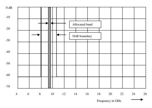
Figure C.4: Maximum permitted spurious emissions power level
