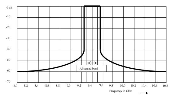
Figure C.3: Maximum permitted out-of-band-emissions power level
