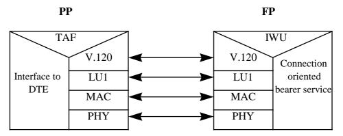
Figure B.2: Profile reference U-plane configuration showing the interworking to a connection-oriented bearer service
