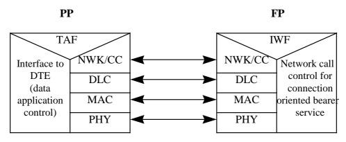
Figure B.3: Profile reference C-plane configuration showing the interworking to the connection-oriented bearer service
