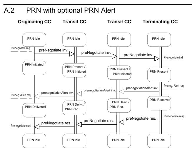
Figure A.2: Example information flow for PRN with optional PRN alert
