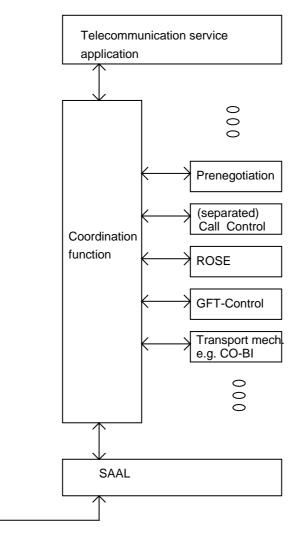
Figure 1: PRN within the B-QSIG/DSS2 protocol model
