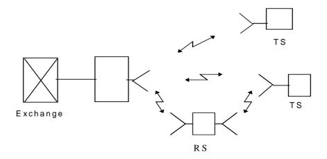
**CS:** Central Station, which is linked to all remote stations (repeater or terminal stations) by microwave transmission paths.
