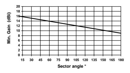
Figure 4: CS sector antenna boresight min gain
