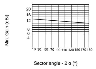
Figure 7: CS central-beam, multi-beam antenna, boresight min gain
