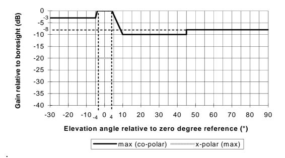
Figure 9: Asymmetric CS antenna elevation patterns
