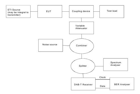
Figure B.2: Bit error performance measurement
