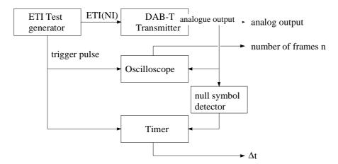
Figure C.2: Measurement of the overall transmitter delay
