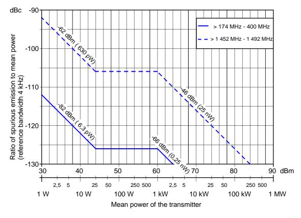
Figure 4.2: Spurious emissions limits for T-DAB transmitters (4 kHz reference bandwidth)
