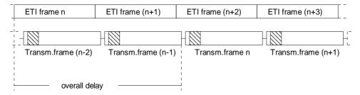
Figure C.1: Overall transmitter delay
