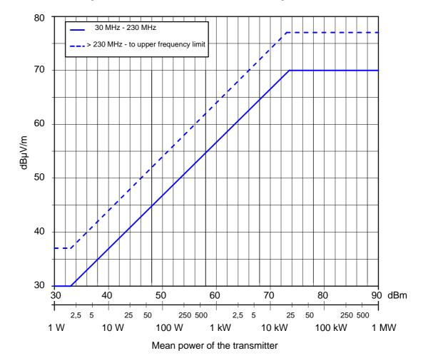
Figure 4.5: Cabinet radiation limits for T-DAB transmitters
