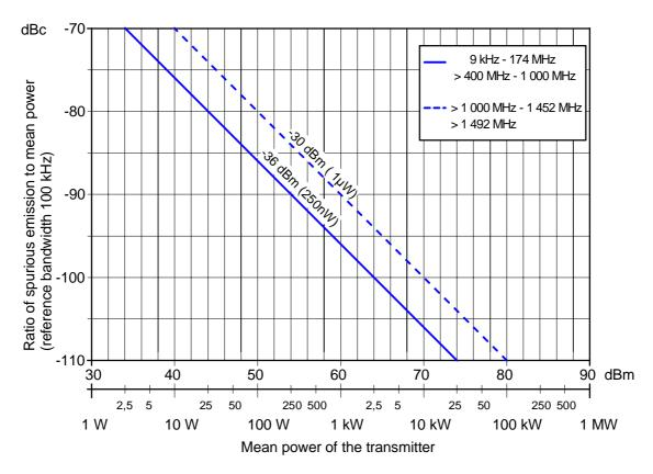
Figure 4.1: Spurious emissions limits for T-DAB transmitters (100 kHz reference bandwidth)
