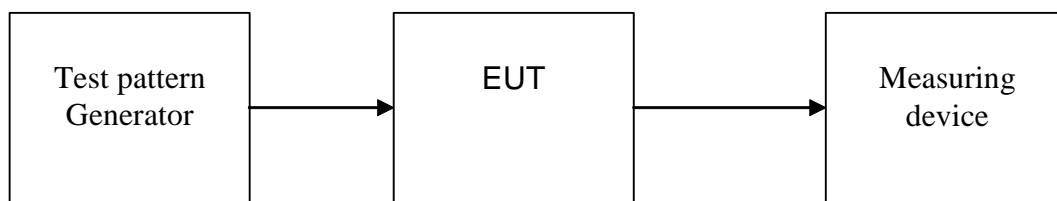
Figure B.1: ETI Test arrangement
