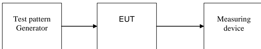
Figure B.1: ETI Test arrangement
