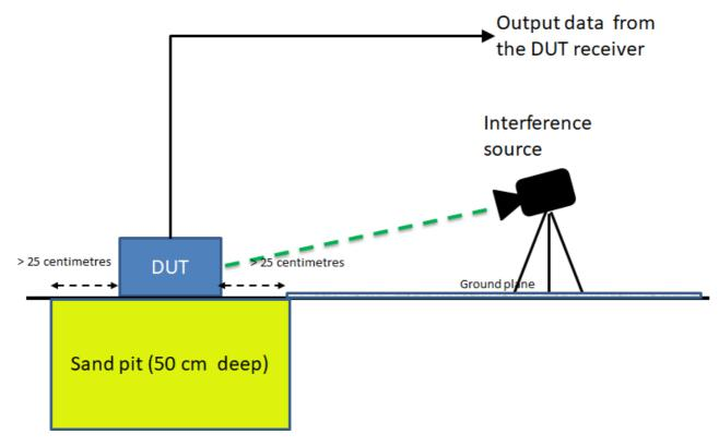
Figure 6: Scenario for receiver testing for large GPR/WPR
