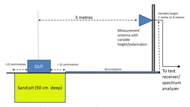
Figure 3: Calibrated setup for large GPR/WPR and measurements below 960 MHz
