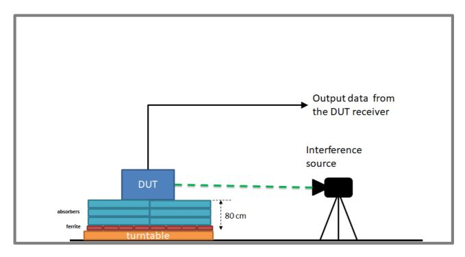
Figure 5: Scenario for receiver testing for small GPR/WPR
