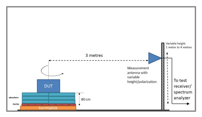
Figure 2: Calibrated setup for small GPR/WPR
