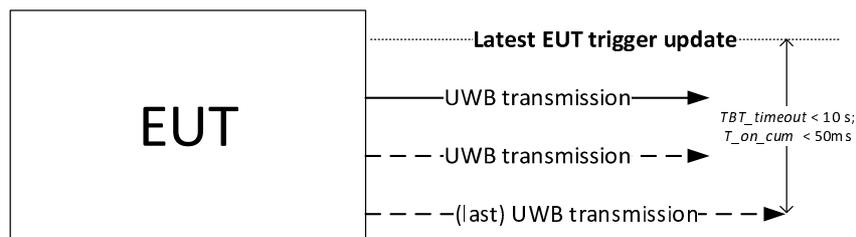
**Figure 4: Trigger-before-transmit limits**
