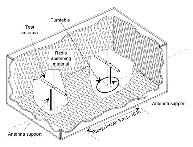
Figure B.1: A typical anechoic chamber
