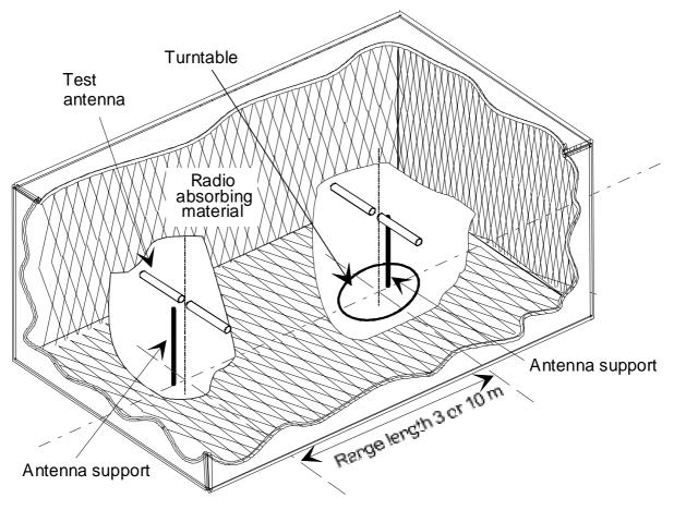
Figure A.1: A typical Anechoic Chamber
