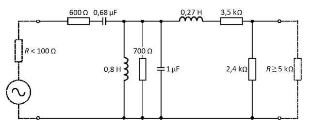
Figure B.3: White Filter circuit
