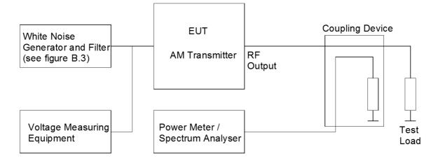
NOTE: In the case of spurious emissions the White Noise Generator and Filter are not used.
