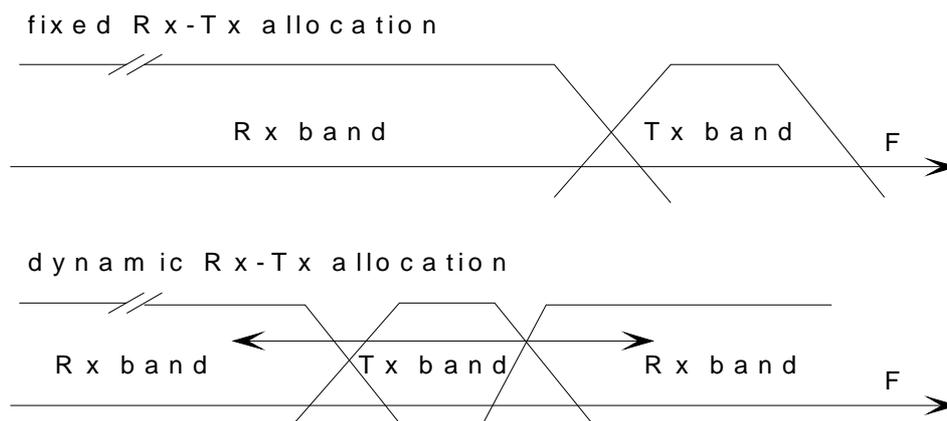
Figure A.2: Possible Frequency Allocation Techniques
