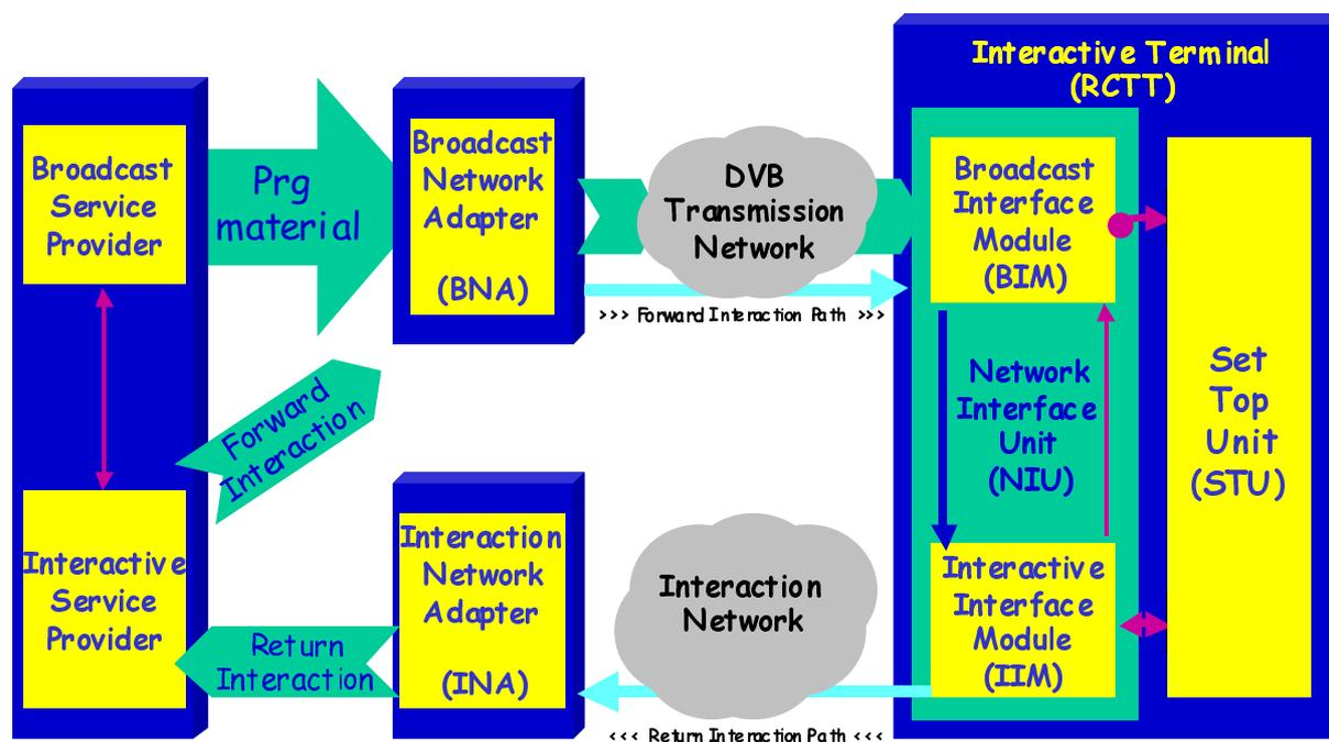
Figure 3: Reference model for terrestrial interactive systems
