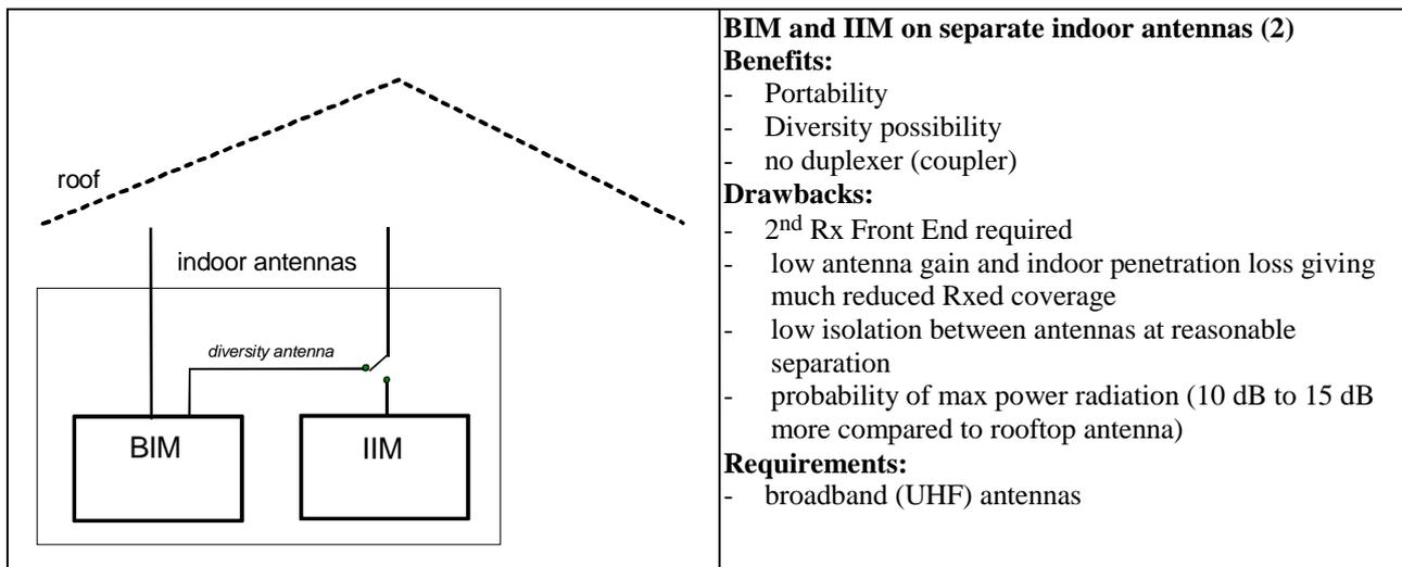
Figure C.1: antenna arrangements
