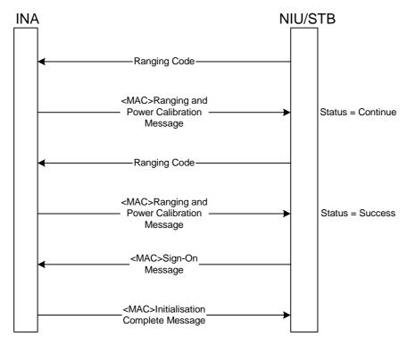
Figure 46: Ranging and Calibration Signalling
