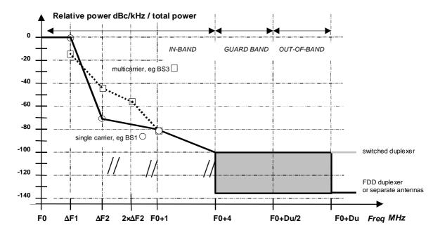
Figure 33: RF transmission power mask
