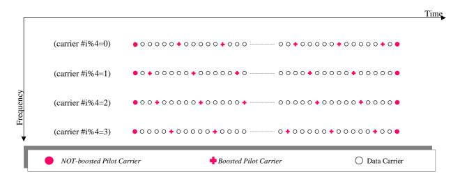
Figure 27: Pilot insertion scheme for the BS2 mini-bursts
