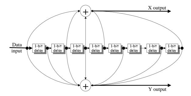
Figure 17: Convolutional Encoder Block diagram
