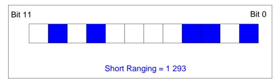
Figure 45: Example of Short/Long ranging sub-channel mapping for MAS1 or MAS2 in 2K mode
