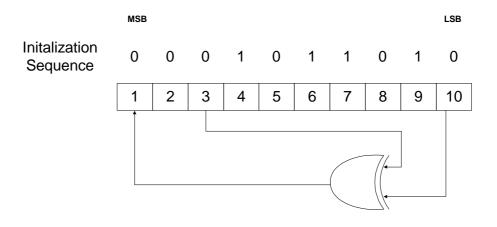
Figure 18: PRBS generator for random interleaving
