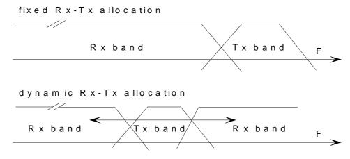
Figure 55: Possible Frequency Allocation Techniques
