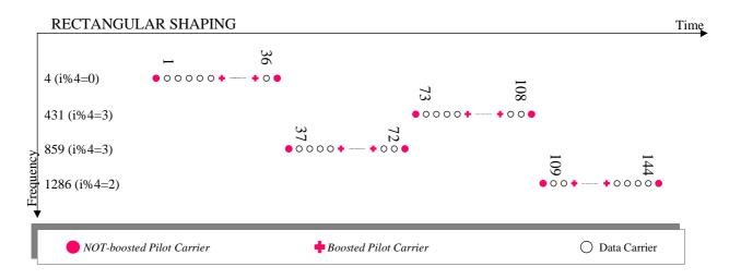
Figure 25: BS1 with frequency hopping and rectangular shaping
