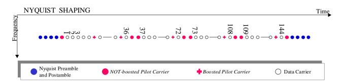
Figure 24: BS1 with Nyquist shaping and without frequency hopping option
