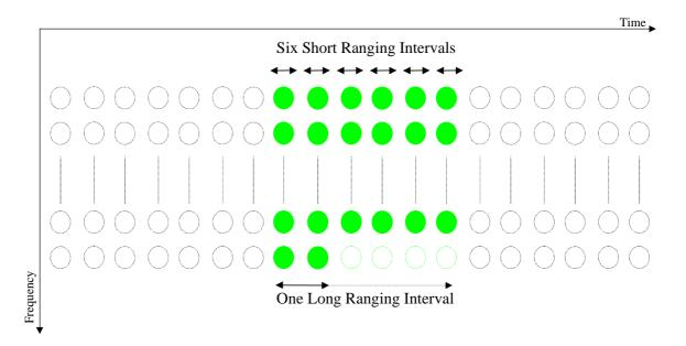
Figure 31: Basic Ranging Interval
