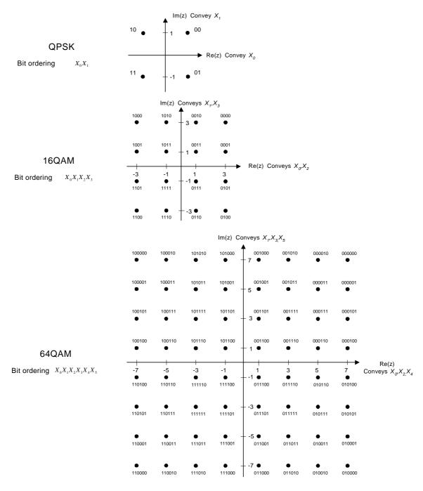
Figure 19: QPSK, 16QAM and 64QAM Constellations
