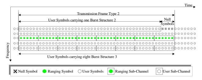
Figure 10: Organization of TF2 frame structure (time domain)
