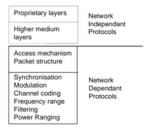
Figure 1: Layer structure for generic system reference model
