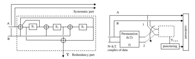
Figure 15: Encoder block diagram (turbo code)
