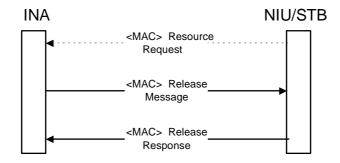
Figure 52: Connection release signalling
