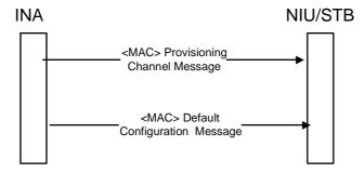
Figure 44: Initialization and Provisioning signalling
