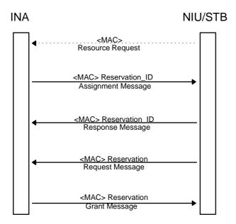
Figure 53: Reservation access signalling
