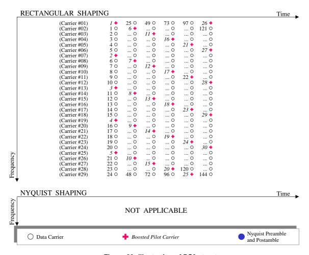
Figure 29: Illustration of BS3 structure
