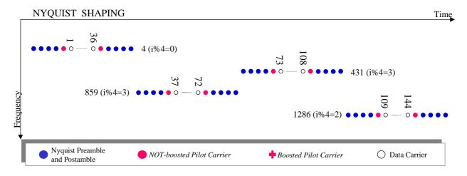
Figure 26: BS1 with frequency hopping and Nyquist shaping
