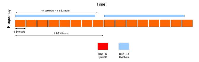
Figure 30: Transmission frame organization for MAS3
