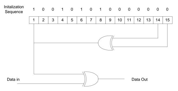
Figure 14: Block diagram for Data Randomization
