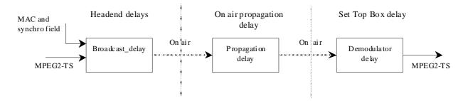
Figure 11: System Model for Timing Analysis
