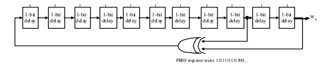
Figure 20: PRBS sequence generator for Pilot modulation
