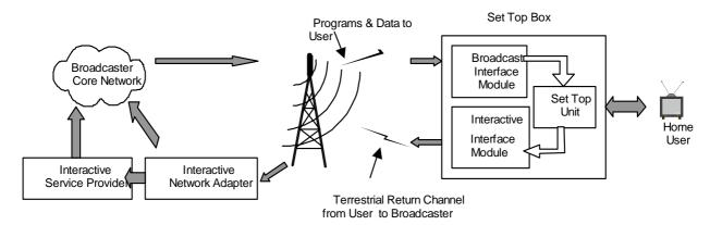
Figure 4: Illustration of the DVB-RCT network
