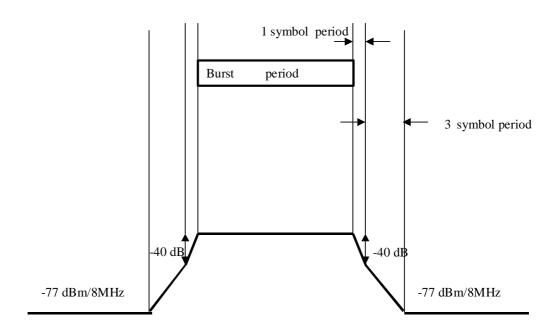
Figure 32: Switching performance of the UHF return channel modulator
