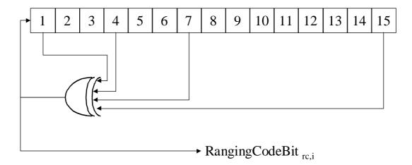
Figure 21: PRBS generator for Ranging Codes
