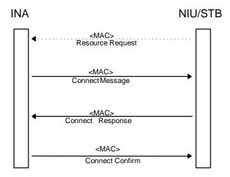
Figure 51: Connection signalling for additional connections
