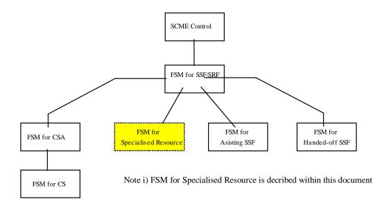
Figure 25: FSM interactions for SCSM-SSF/SRF
