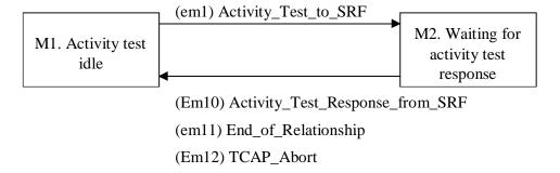
Figure 23: Activitytest FSM
