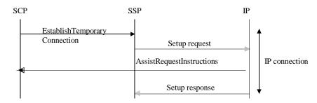
Figure 6: Connection to IP with direct link to SCP, IP initiates interaction with SCP
