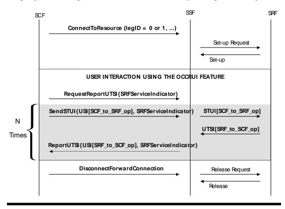
Figure 10: User Interaction in the SRF relay case: OCCRUI mechanism
