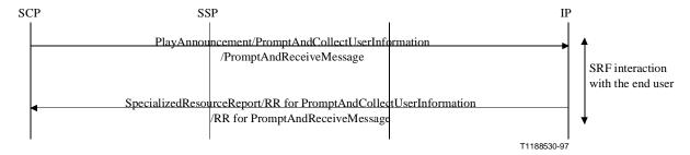
Figure 12: Direct SCF-SRF of user interaction operations and responses
