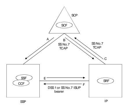
Figure 19: Direct SCP-IP information transfer
