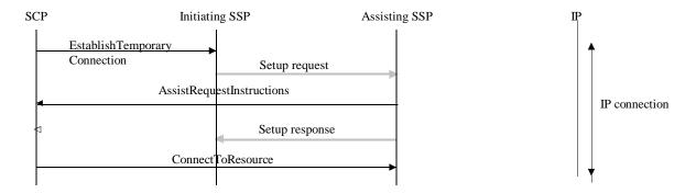
Figure 7: Preamble for assist case with integrated IP or external IP and SSP relay of SCP-IP messages
