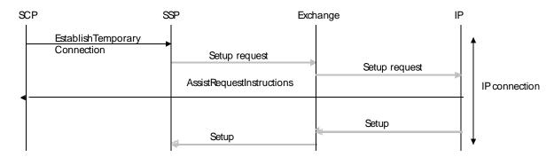
Figure 8: Preamble for assist case with external IP and direct SCP-IP messaging
