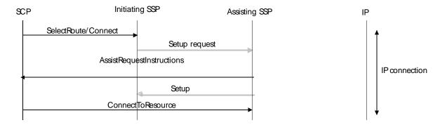
Figure 9: Preamble for hand-off case
