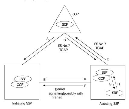
Figure 20: SSP assist(relay SSP)
