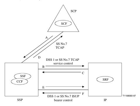
Figure 18: SSP relays messages between SCP and IP
