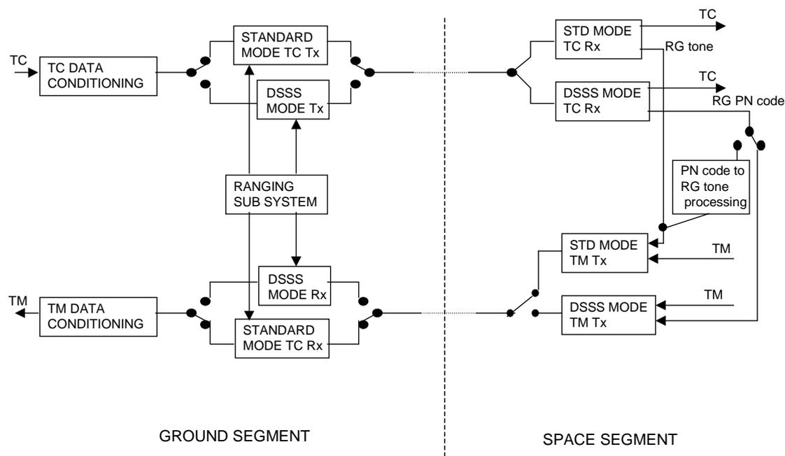
Figure 4: Generic system functional block diagram
