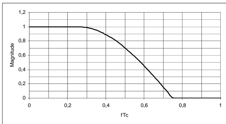
Figure D.1: SRRC frequency response for Alpha = 0,5
