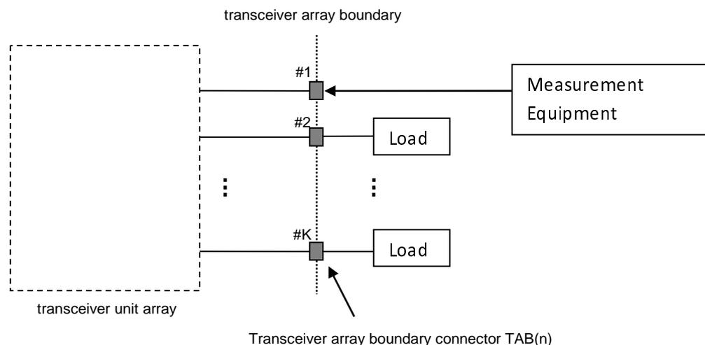
**Figure C.2: Receiver test ports**
