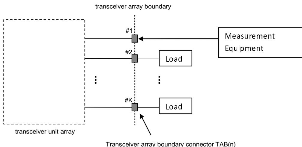
**Figure C.1: Transmitter test ports**
