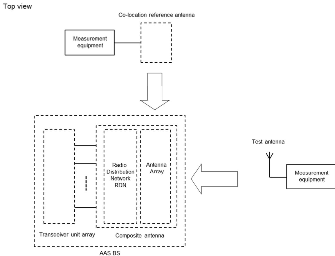
**Figure D.4: Receiver test interfaces for co-location concept**
