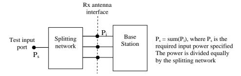
Figure B.5.1-1: Receiver test set-up
