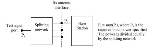
Figure B.5.1-1: Receiver test set-up
