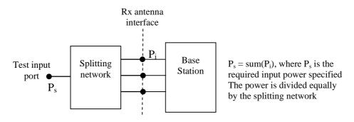
Figure B.5.1-1: Receiver test set-up
