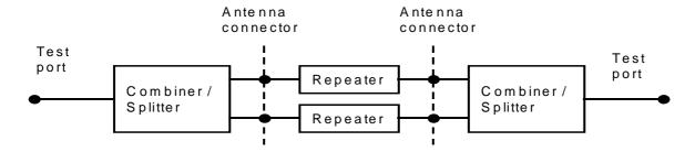
Figure B.3-1: Example of Repeater configuration
